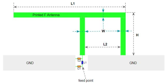
• Antenna ref. sizes: L1=26.5mm / L2=5mm / H=7.4mm / W=1mm
