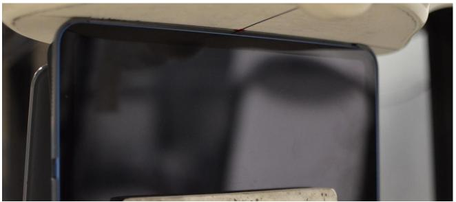
SAR Test Setup Photo 2: Body, Tablet (FCC ID: BCGA2696) with Keyboard Accessory Case, Left Edge, 0 mm
