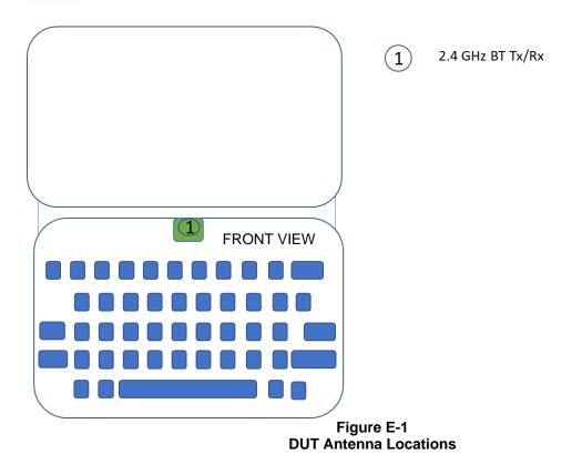
Note: Exact antenna dimensions and separation distances are shown in the Technical Descriptions in the FCC Filing.
