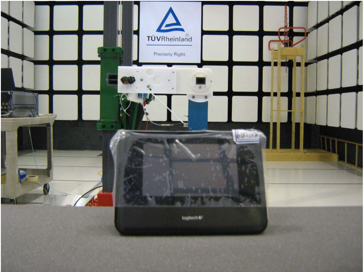
Figure 4: Photo of Test Setup for X-RC4, 18 GHz to 26GHz (Rear View)
