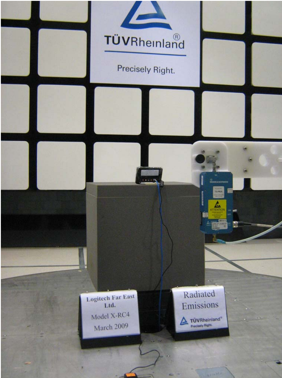
Figure 3: Photo of Test Setup for X-RC4, 18 GHz to 26GHz (Front View)
