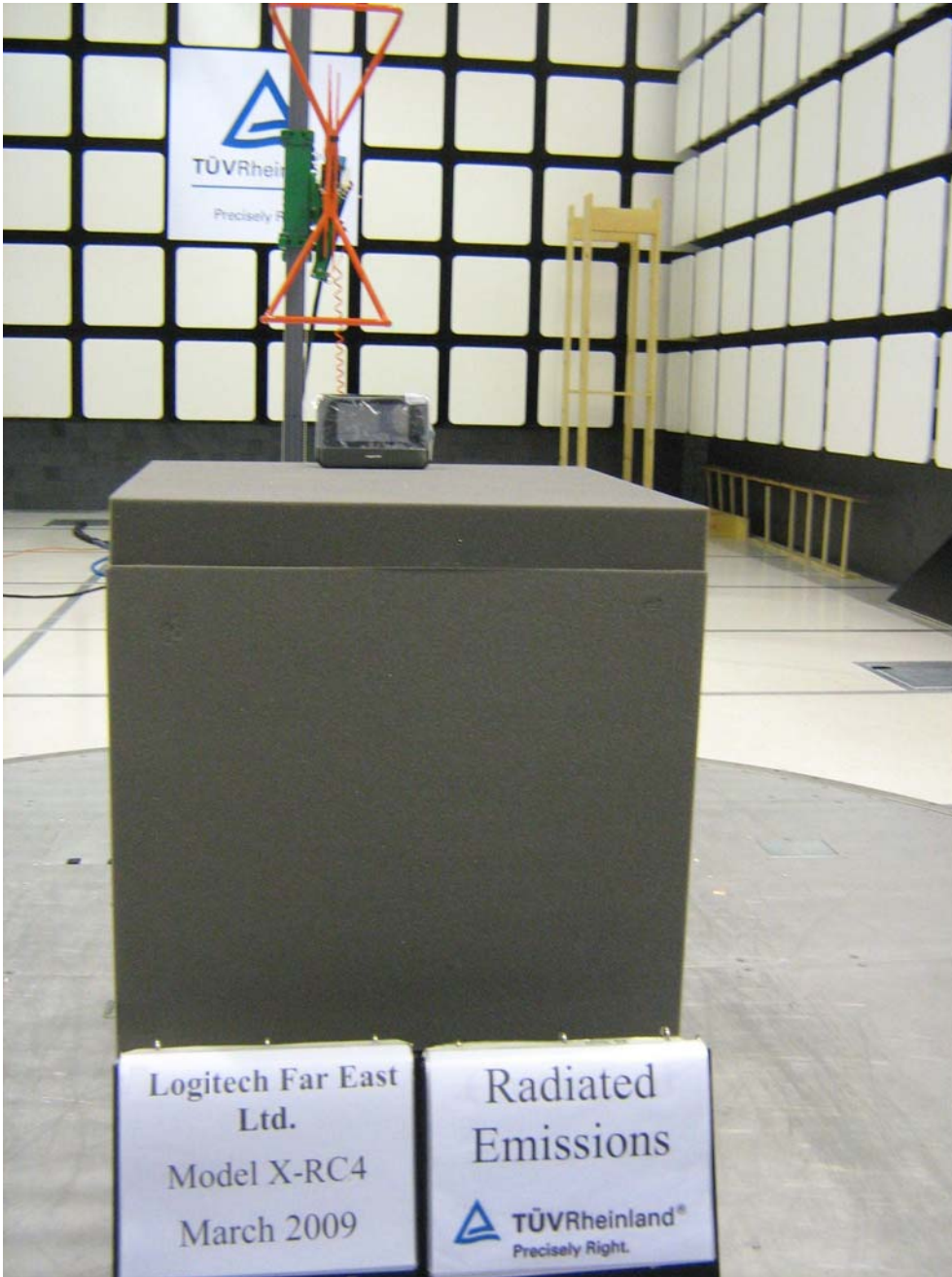
Figure 2: Photo of Test Setup for X-RC4, 30 to 1000 MHz (Rear View)
