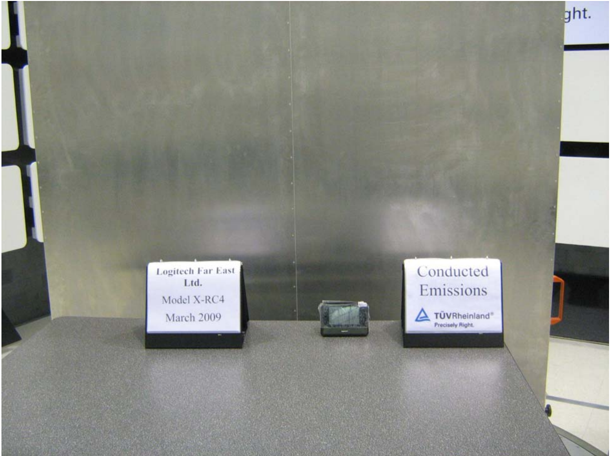
Figure 5: Photo of Test Setup for X-RC4, AC Conducted Emission (Front View)
