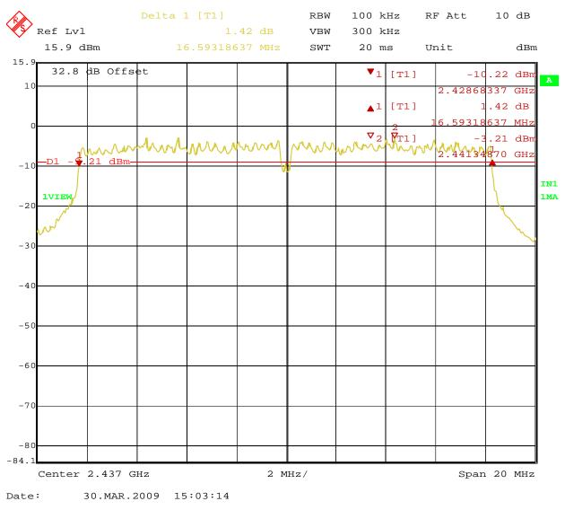
Figure 16: 6dB Bandwidth at 54Mbit/s – Operating Channel 2437 MHz (Vertical)
