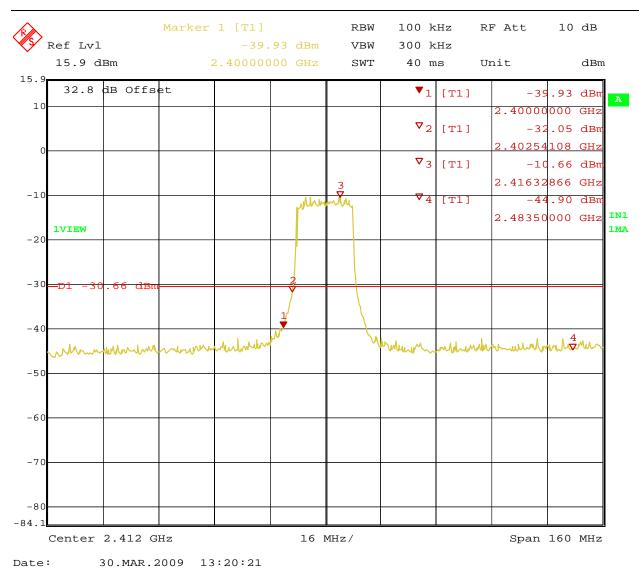
Figure 31: Band-edge Requirement for Operating Channel 2412 MHz (Horizontal)
