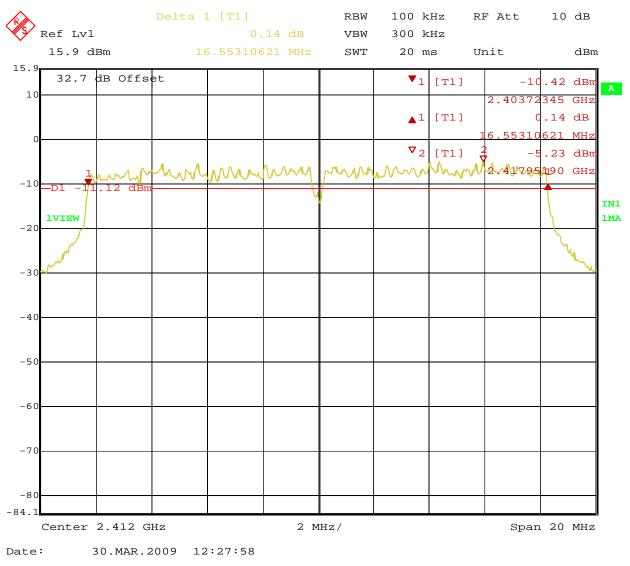
Figure 14: 6dB Bandwidth at 54Mbit/s – Operating Channel 2412 MHz (Vertical)
