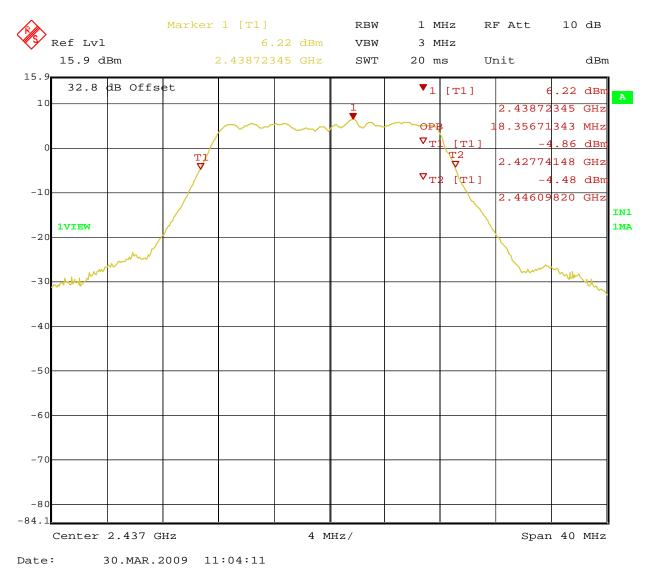
Figure 28: 99% Bandwidth at 54Mbit/s – Operating Channel 2437 MHz (Vertical)
