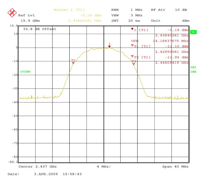
Figure 21: 99% Bandwidth at 11Mbit/s – Operating Channel 2437 MHz (Horizontal)
