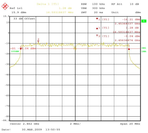
Figure 17: 6dB Bandwidth at 54Mbit/s – Operating Channel 2462 MHz (Horizontal)
