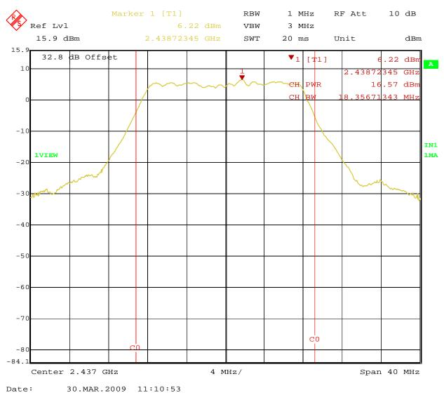
Figure 4: Maximum Transmitted Power at 3 Meter – Middle Channel 2437 MHz (Vertical)
