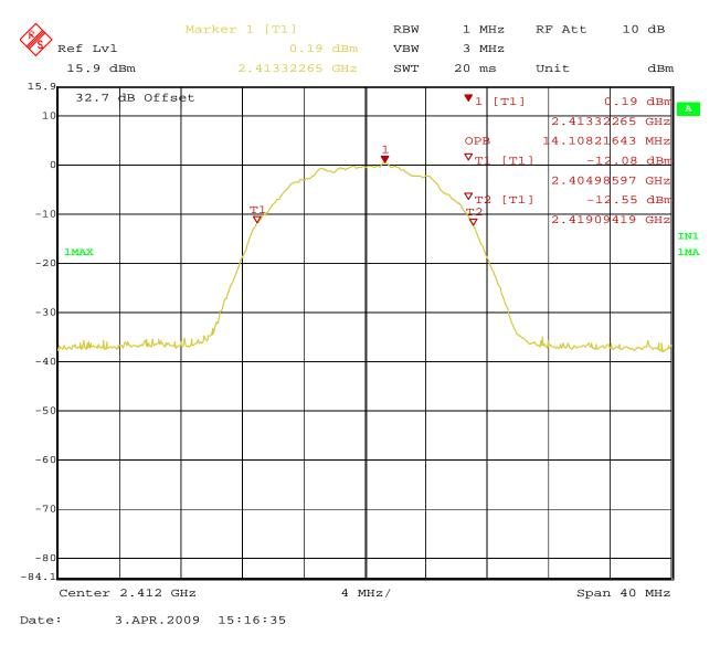
Figure 19: 99% Bandwidth at 11Mbit/s – Operating Channel 2412 MHz (Horizontal)
