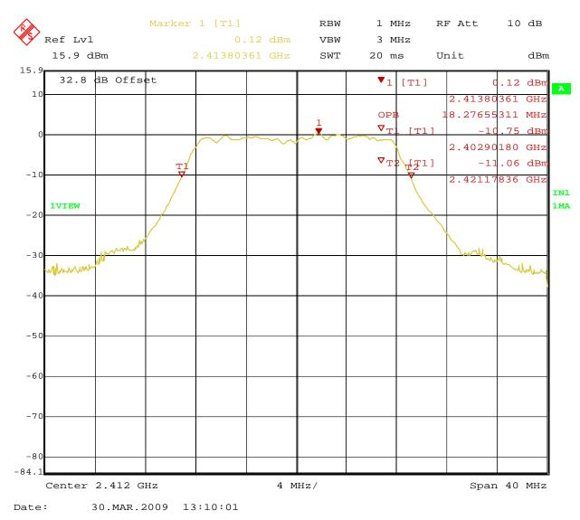
Figure 25: 99% Bandwidth at 54Mbit/s – Operating Channel 2412 MHz (Horizontal)
