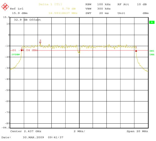
Figure 15: 6dB Bandwidth at 54Mbit/s – Operating Channel 2437 MHz (Horizontal)
