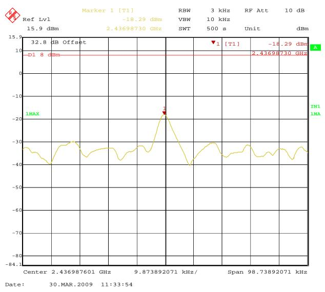
Figure 40: Peak Power Spectral Density for Operating Channel 2437MHz (Vertical)
