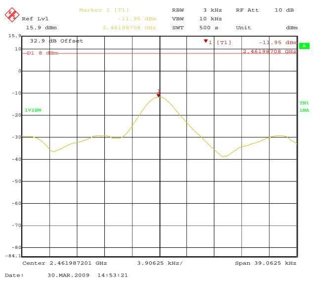
Figure 42: Peak Power Spectral Density for Operating Channel 2462MHz (Vertical)
