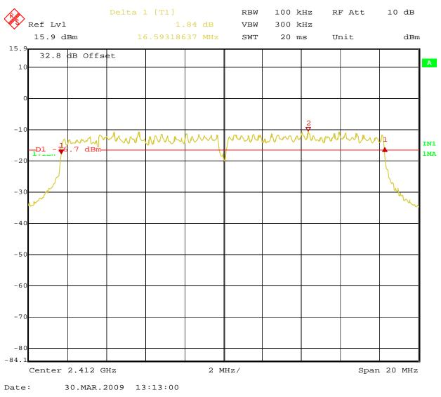
Figure 13: 6dB Bandwidth at 54Mbit/s – Operating Channel 2412 MHz (Horizontal)
