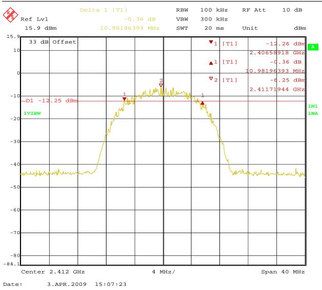
Figure 7: 6dB Bandwidth at 11Mbit/s – Operating Channel 2412 MHz (Horizontal)
