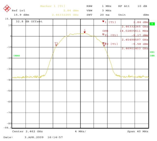
Figure 23: 99% Bandwidth at 11Mbit/s – Operating Channel 2462 MHz (Horizontal)
