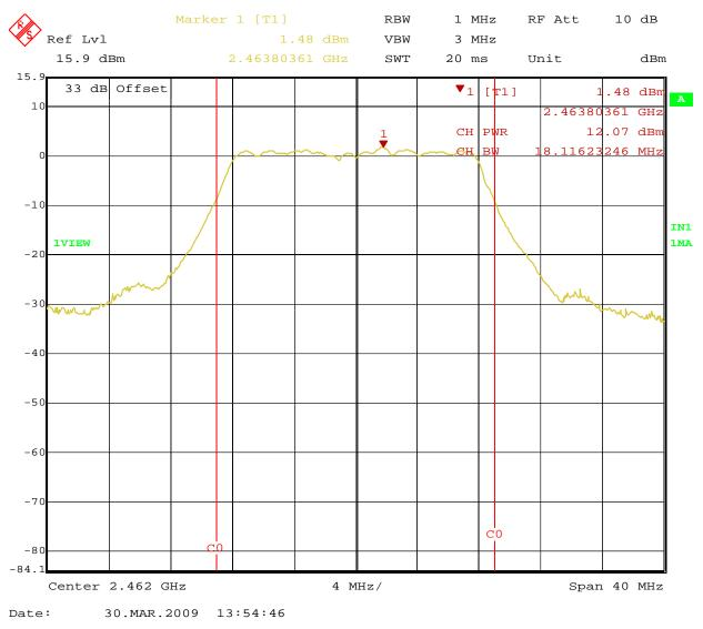
Figure 5: Maximum Transmitted Power at 3 Meter – Highest Channel 2462 MHz (Horizontal)
