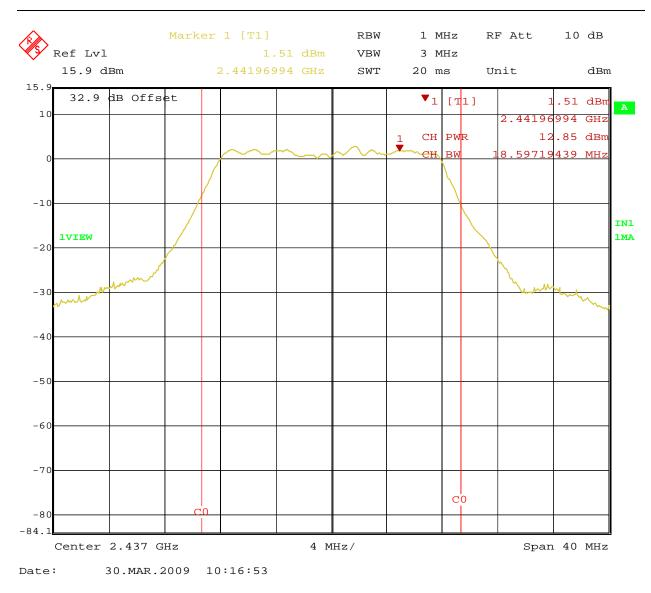
Figure 3: Maximum Transmitted Power at 3 Meter – Middle Channel 2437 MHz (Horizontal)
