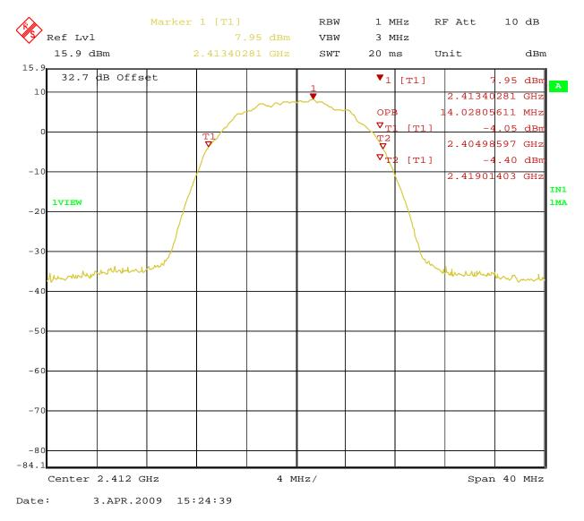
Figure 20: 99% Bandwidth at 11Mbit/s – Operating Channel 2412 MHz (Vertical)
