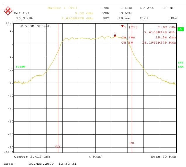
Figure 2: Maximum Transmitted Power at 3 Meter – Lowest Channel 2412 MHz (Vertical)
