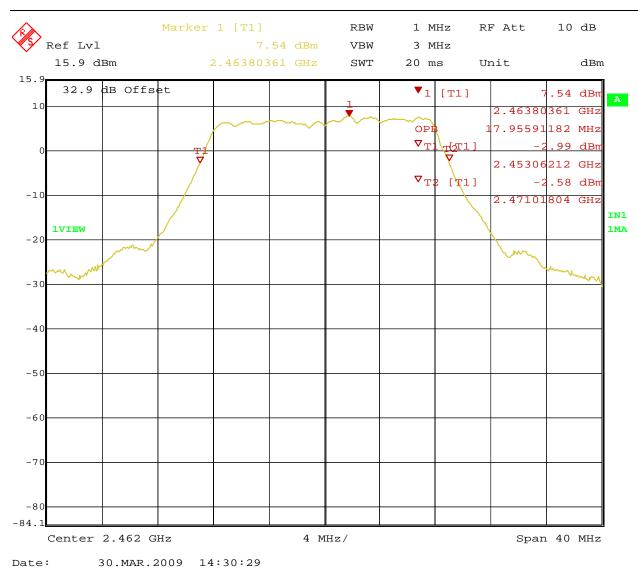
Figure 30: 99% Bandwidth at 54Mbit/s – Operating Channel 2462 MHz (Vertical)
