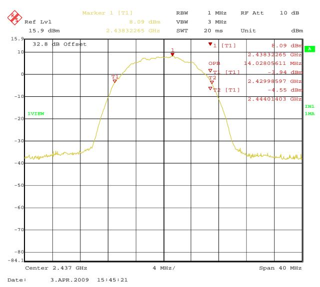
Figure 22: 99% Bandwidth at 11Mbit/s – Operating Channel 2437 MHz (Vertical)
