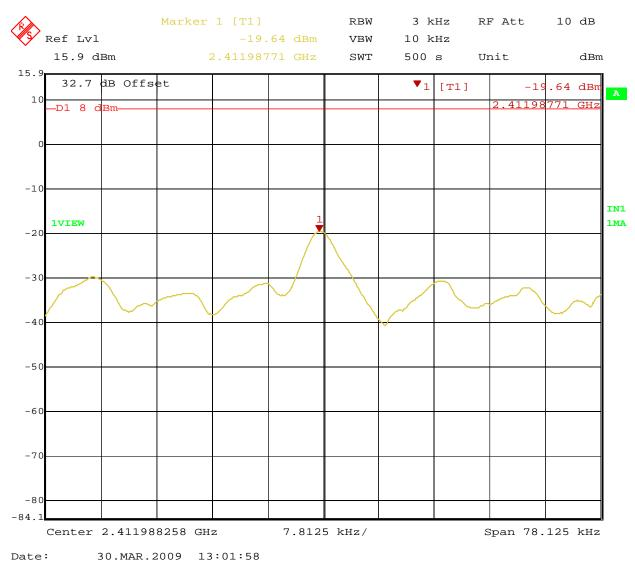
Figure 38: Peak Power Spectral Density for Operating Channel 2412MHz (Vertical)
