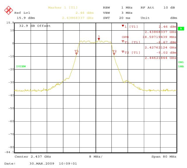
Figure 27: 99% Bandwidth at 54Mbit/s – Operating Channel 2437 MHz (Horizontal)
