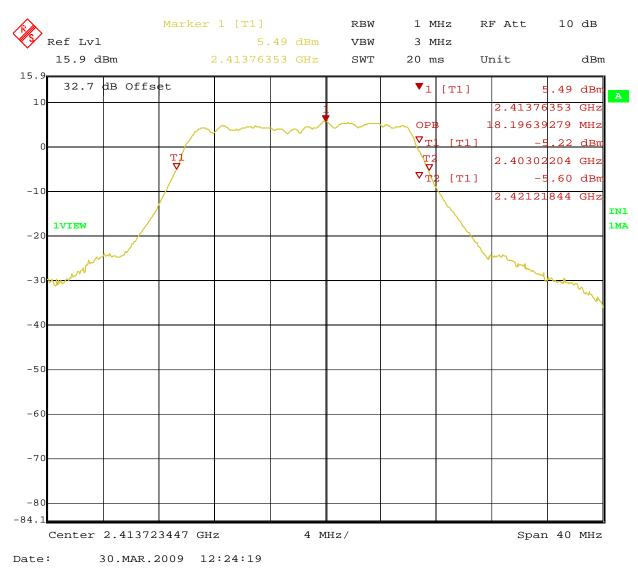
Figure 26: 99% Bandwidth at 54Mbit/s – Operating Channel 2412 MHz (Vertical)
