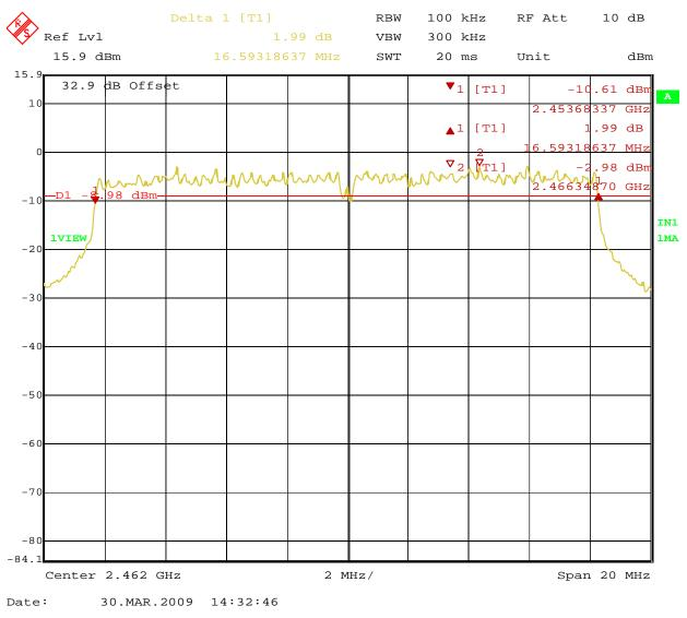
Figure 18: 6dB Bandwidth at 54Mbit/s – Operating Channel 2462 MHz (Vertical)
