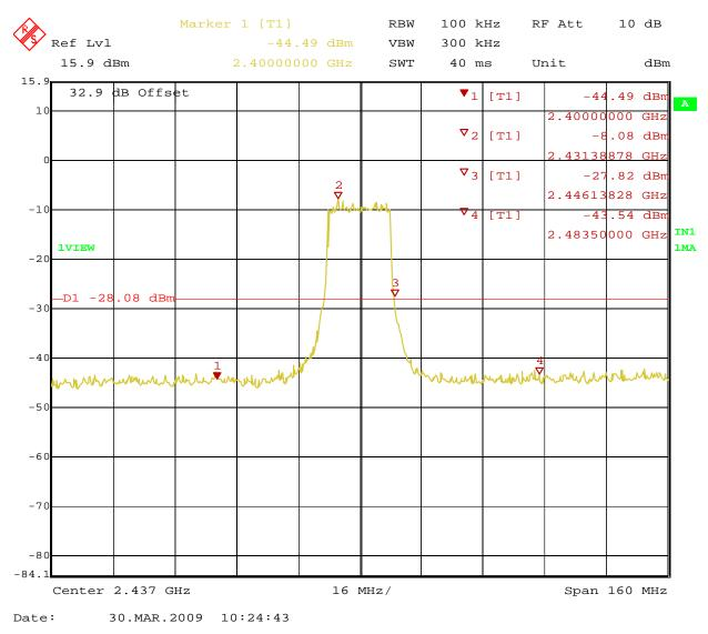
Figure 33: Band-edge Requirement for Operating Channel 2437MHz (Horizontal)
