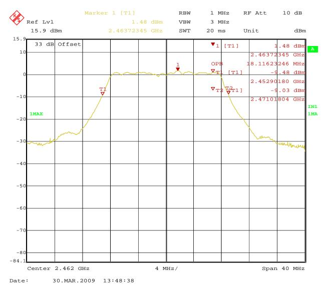
Figure 29: 99% Bandwidth at 54Mbit/s – Operating Channel 2462 MHz (Horizontal)
