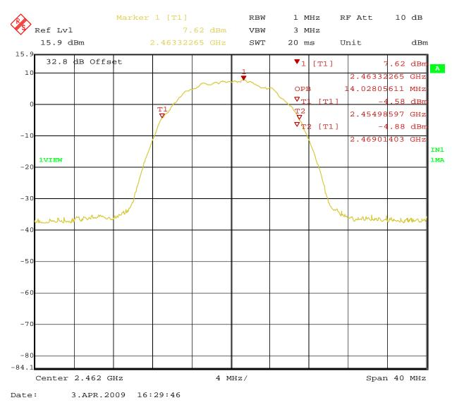
Figure 24: 99% Bandwidth at 11Mbit/s – Operating Channel 2462 MHz (Vertical)
