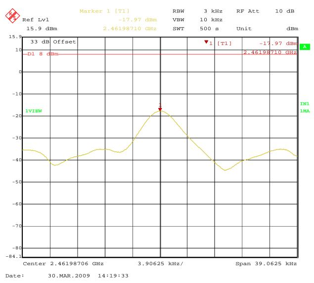
Figure 41: Peak Power Spectral Density for Operating Channel 2462MHz (Horizontal)
