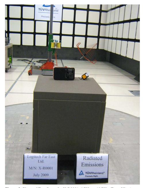
Figure 3: Photo of Test Setup for X-R0001, 1GHz to 18GHz (Front View)
