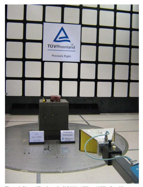
Figure 4: Photo of Test Setup for X-R0001, 1GHz to 18GHz (Rear View)
