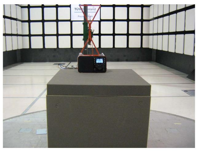
Figure 1: Photo of Test Setup for X-R0001, 30 MHz to 1000MHz (Front View)
