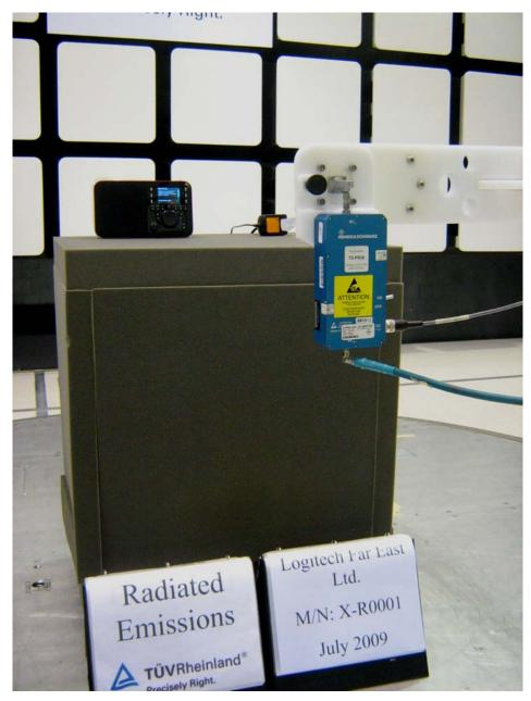
Figure 5: Photo of Test Setup for X-R0001, 18 GHz to 26GHz (Front View)
