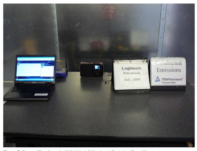
**Figure 7:** Photo of Test Setup for X-R0001, AC Conducted Emission (Front View)
