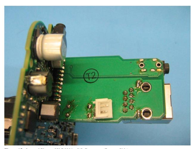
**Figure 15:** Internal Photo of X-R0001 – I/O Connector (Bottom Side)
