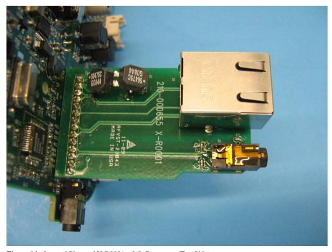
**Figure 14:** Internal Photo of X-R0001 – I/O Connector (Top Side)
