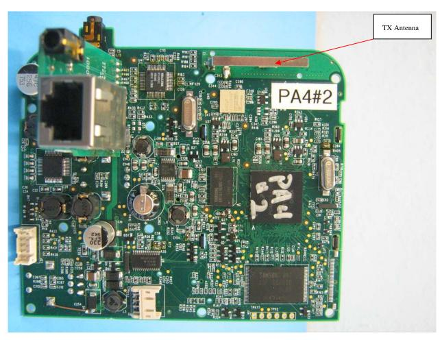
Figure 13: Internal Photo of X-R0001 - PCB Board (Rear Side)
