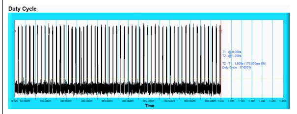
**NOTE:** T1 denotes the start of duty cycle period is  $0^{th}$  second. T2 denotes the end of duty cycle period is  $1^{th}$  second. T2 – T1= 1 seconds. Duty Cycle = 17.650%
