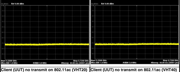
Client (UUT) no transmit on 802.11ac (VHT20) mode
