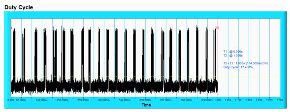
**NOTE:** T1 denotes the start of duty cycle period is  $0^{th}$  second. T2 denotes the end of duty cycle period is  $1^{th}$  second. T2 – T1= 1 seconds. Duty Cycle = 17.450%
