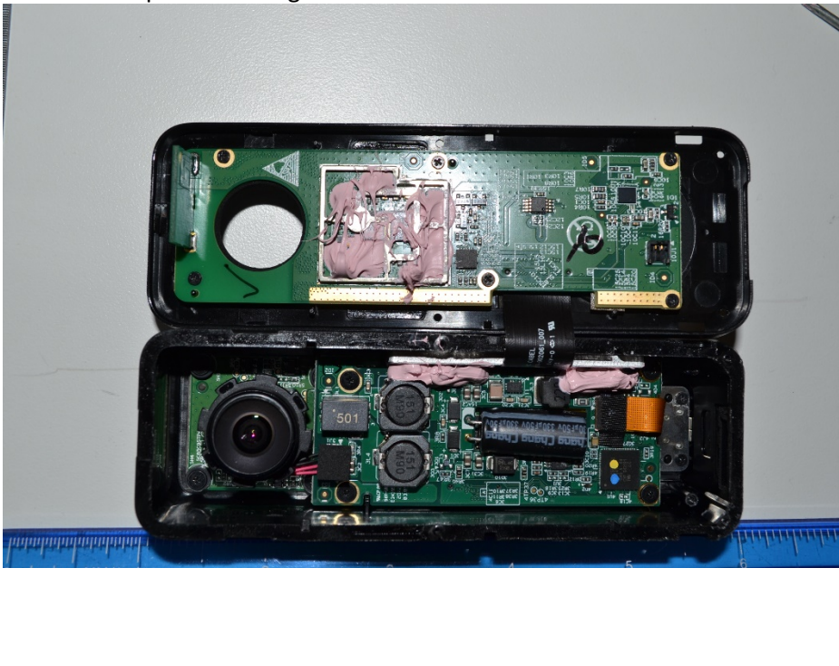
EUT radio chip set shielding removed
