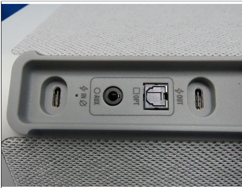
Difference (Change the DC-in Jack and Charge-out port to USB-C)
