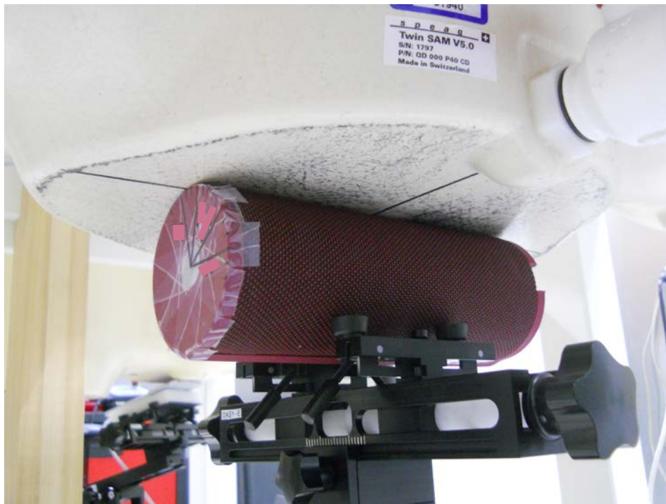
Test Setup Photo 6: Side at 0.0 mm (5 GHz WLAN Chain0)
