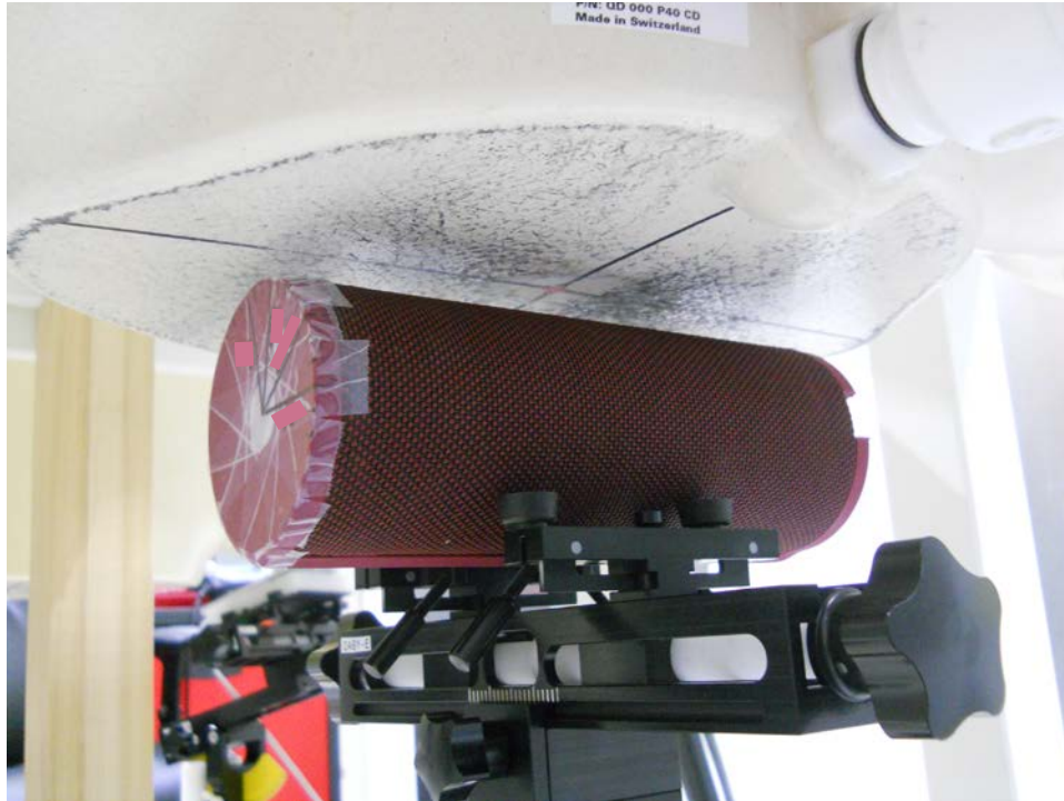
Test Setup Photo 5: Side at 1.0 mm (5 GHz WLAN Chain0)
