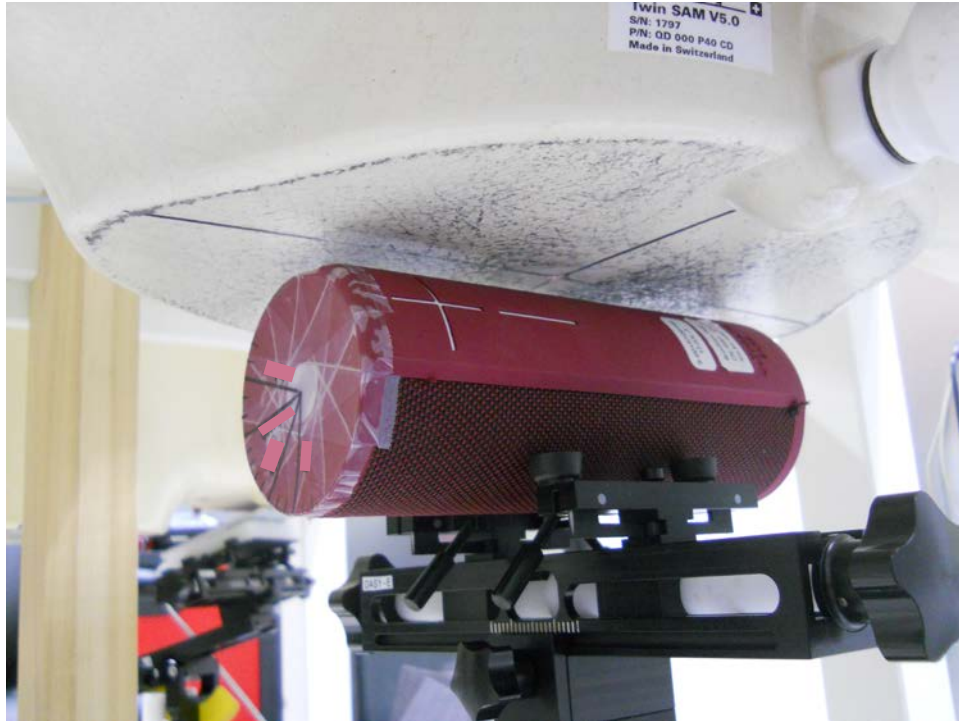
Test Setup Photo 9: Side at 1.0 mm (Bluetooth)
