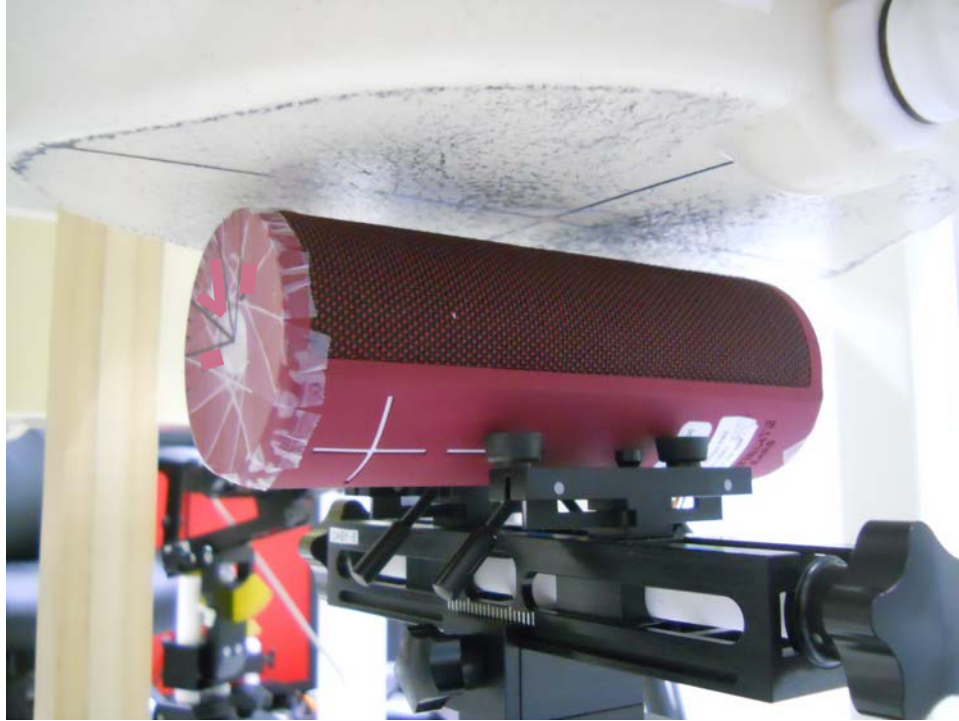
Test Setup Photo 7: Side at 1.0 mm (5 GHz WLAN Chain1)
