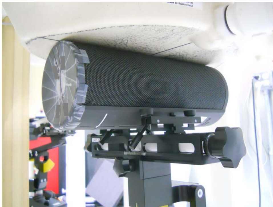
Test Setup Photo 4: Side at 0.0 cm (2.4 GHz WLAN Chain1)
