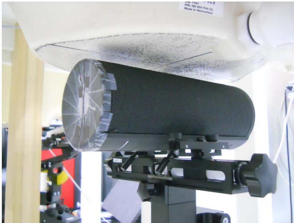
Test Setup Photo 7: Side at 1.0 cm (5 GHz WLAN Chain1)
