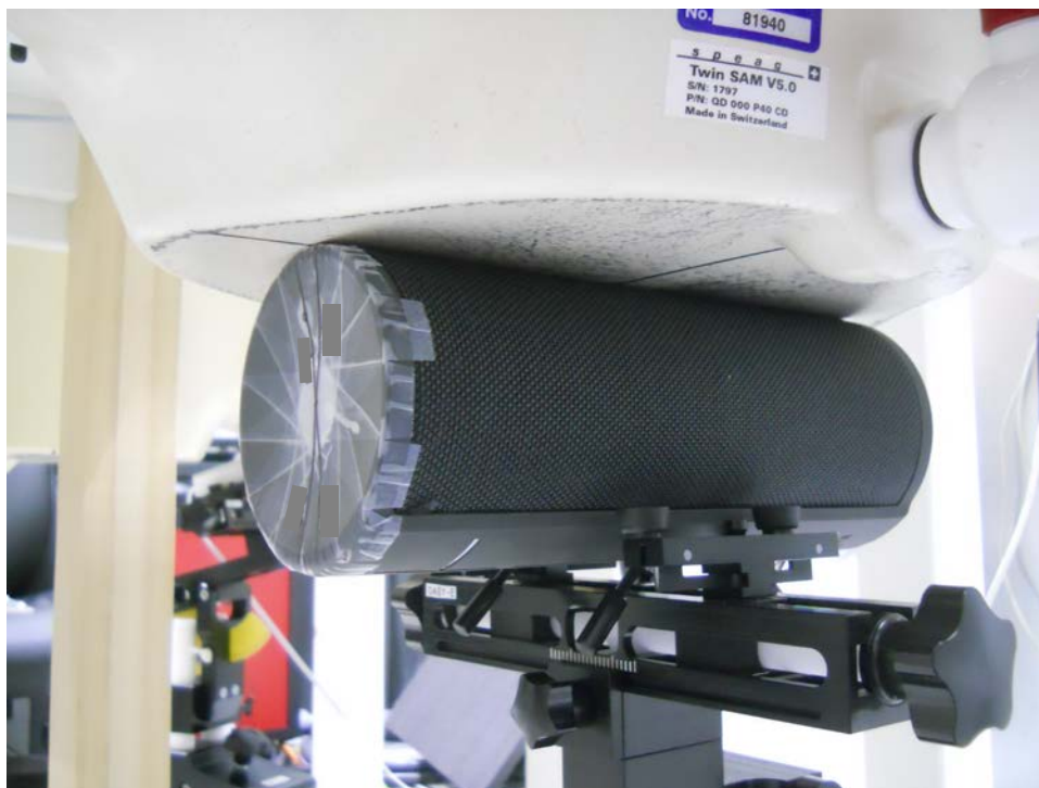
Test Setup Photo 8: Side at 0.0 cm (5 GHz WLAN Chain1)
