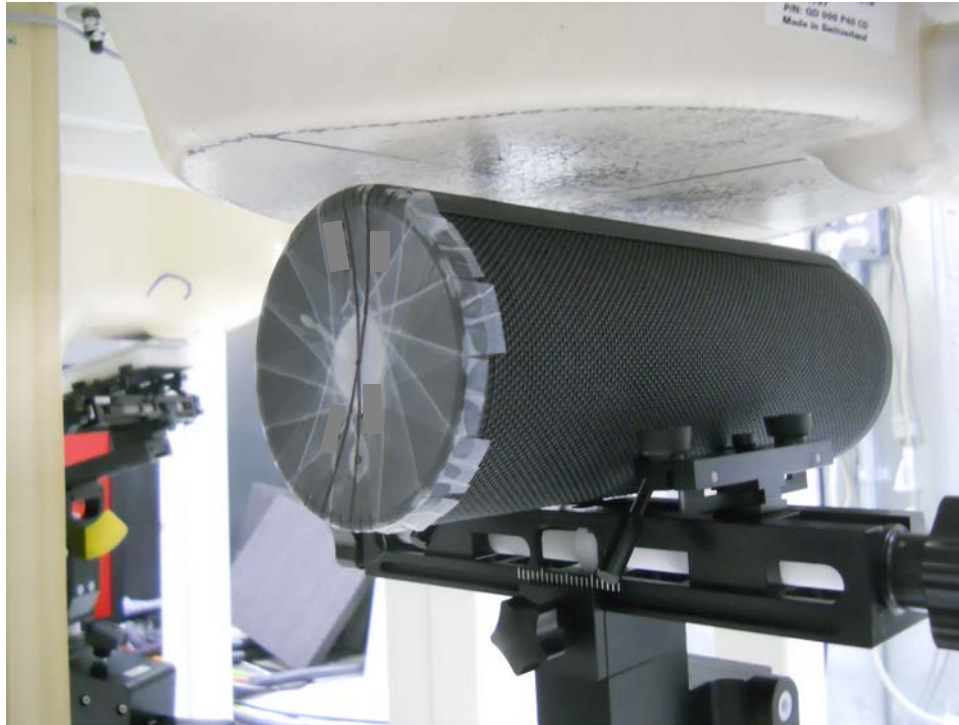
Test Setup Photo 1: Side at 1.0 cm (2.4 GHz WLAN Chain0)
