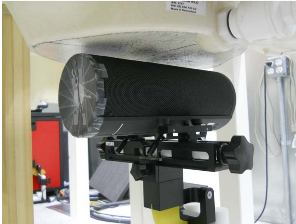
Test Setup Photo 3: Side at 1.0 cm (2.4 GHz WLAN Chain1)
