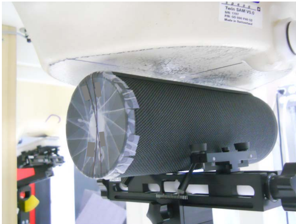
Test Setup Photo 5: Side at 1.0 cm (5 GHz WLAN Chain0)
