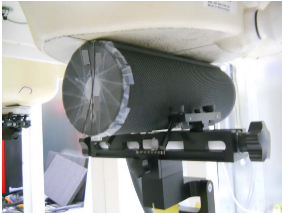
Test Setup Photo 2: Side at 0.0 cm (2.4 GHz WLAN Chain0)
