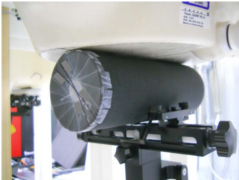
Test Setup Photo 10: Side at 0.0 cm (Bluetooth)
