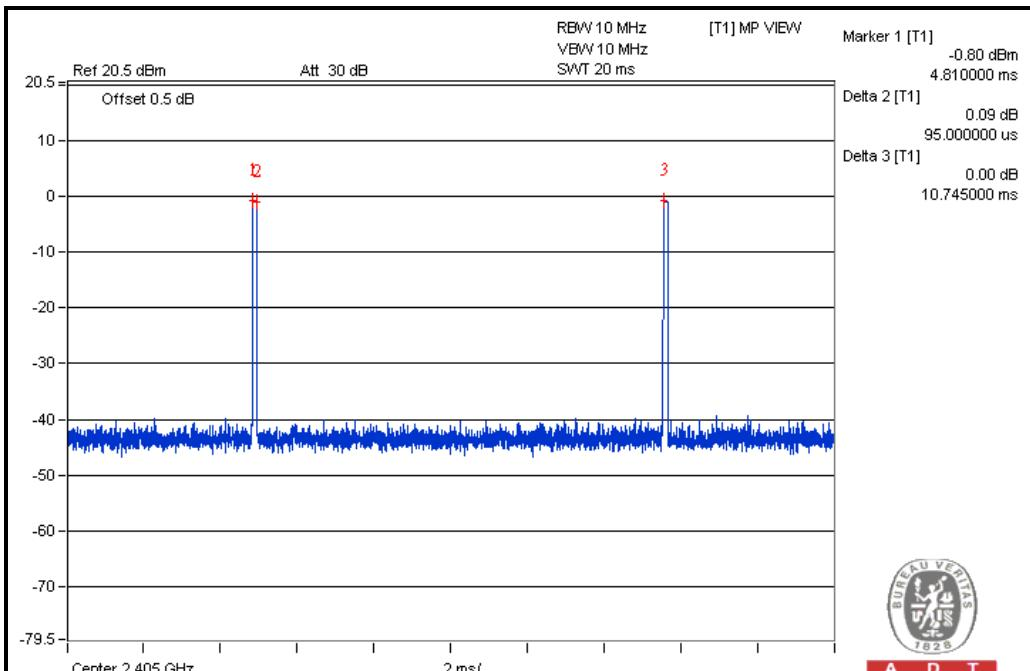
$$20 \log (\text{Duty cycle}) = 20 \log (0.095 \text{ ms} / 10.745 \text{ ms}) = -41.1 \text{ dB}$$
