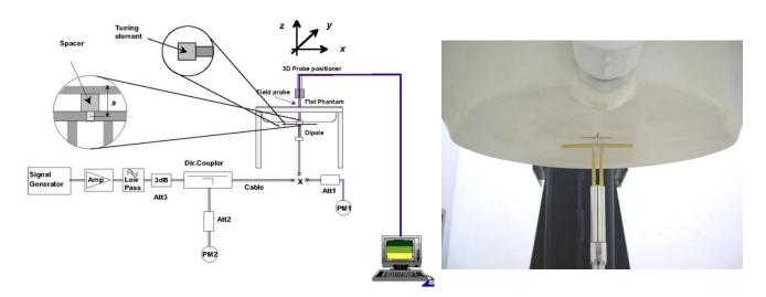
Fig 8.3.1 System Performance Check Setup
