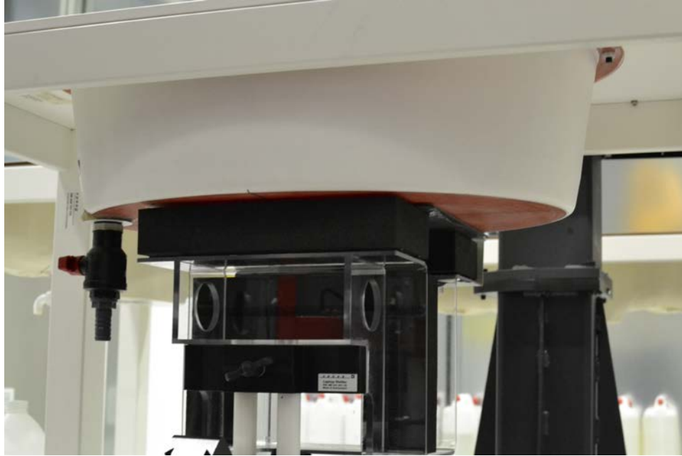
SAR Test Setup Photo 1 – Top Side at 0 mm
