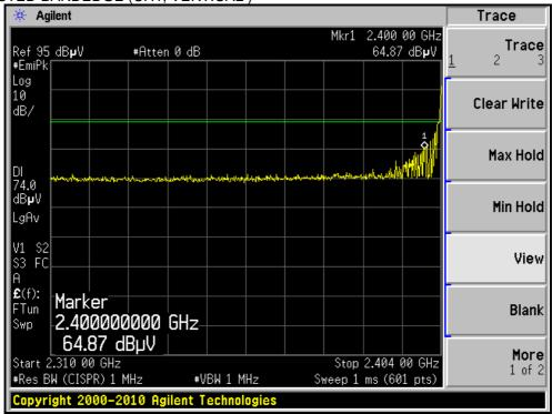
\* The average value of fundamental frequency is: Average = Peak value + 20log(Duty cycle). And it meets the requirement of limit.
