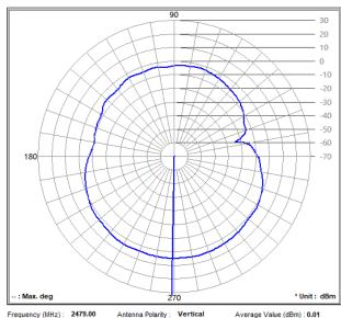
Frequency (MHz): 2479.00 Antenna Polarity: Vertical
