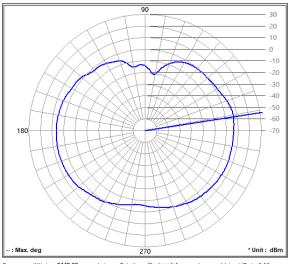
Average Value (dBm): 3.06 Frequency (MHz): 2442.00 Antenna Polarity: Horizontal
