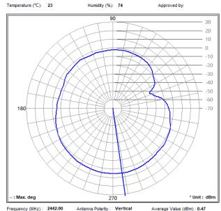
Frequency (MHz): 2442.00 Antenna Polarity: Vertical
