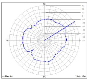
Frequency (MHz): 2403.00 Antenna Polarity: Horizontal Average Value (dBm): -9.03
