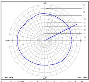
Average Value (dBm) : 4.30 Frequency (MHz): 2442.00 Antenna Polarity: Horizontal
