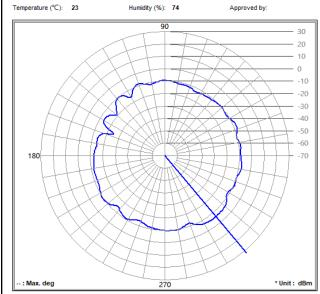
Frequency (MHz): 2442.00 Antenna Polarity: Vertical Average Value (dBm) : -10.26
