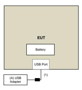
For AC Power Conducted Emission test
