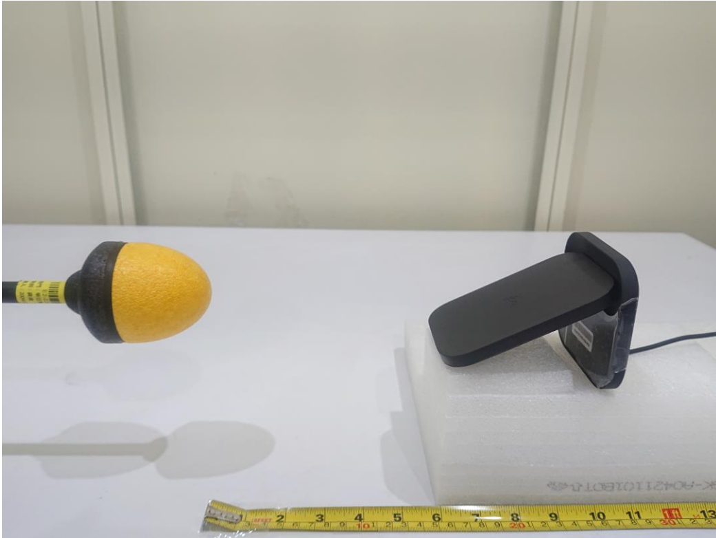
E-Field (Standby Mode – Z-axis)
