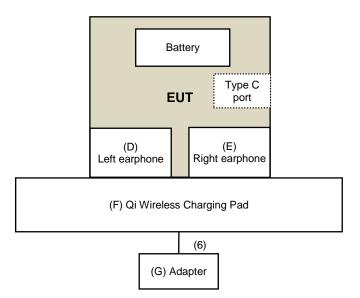
For radiated emission bleow 1GHz test:
