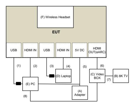
For Unwanted Emission (above 1GHz) test
