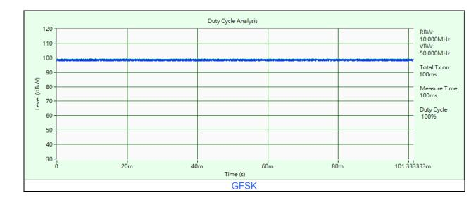
GFSK: Duty cycle = 100 ms / 100 ms x 100% = 100.0%
