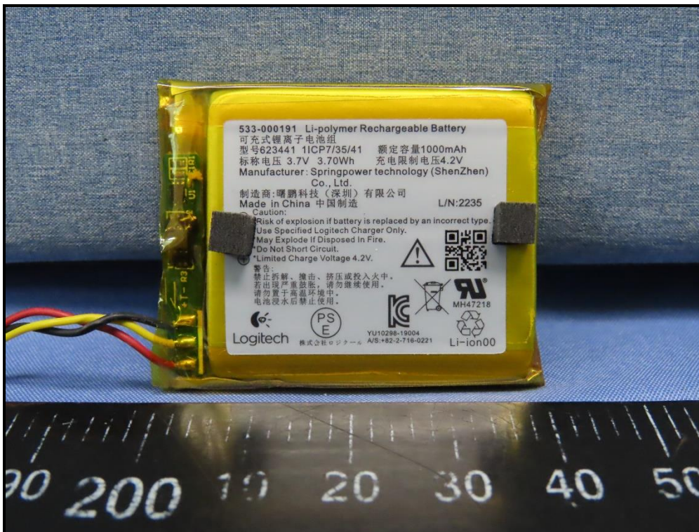
Battery (Brand: Springpower technology (ShenZhen) Co.,Ltd.; Model: 533-000191 or 623441)
