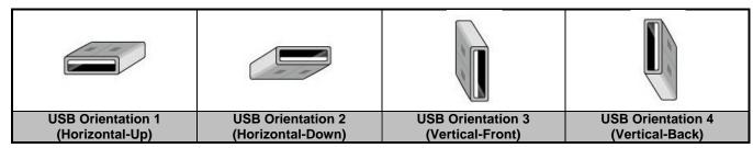
Fig-4.1 Illustration for USB Connector Orientations
