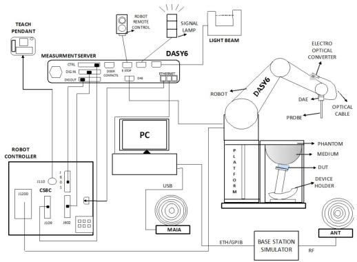
Fig-3.1 SPEAG DASY6 System Setup
