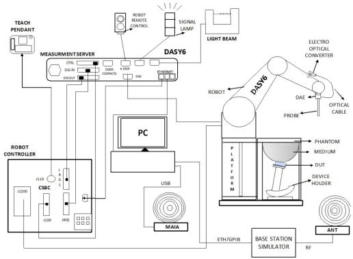
Fig-3.1 SPEAG DASY6 System Setup
