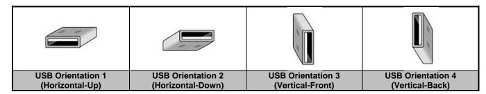
Fig-4.1 Illustration for USB Connector Orientations
