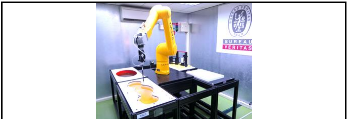
Fig-3.2 SPEAG DASY6 System
