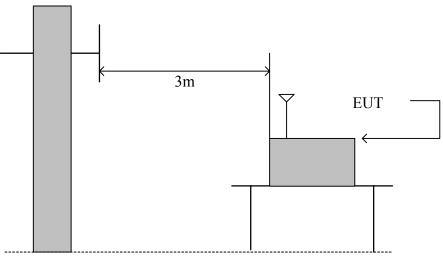
Antenna Elevation Variable
