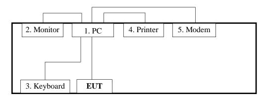
Both conducted and radiated testing were performed according to the procedures in ANSI C63.4: 1992. Radiated testing was performed at an antenna to EUT distance of 10 m on an open area test site. Please refer to the photos of test configuration in Item 5.
