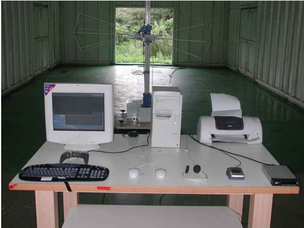
Front View of Radiated Test (BiconiLog)
