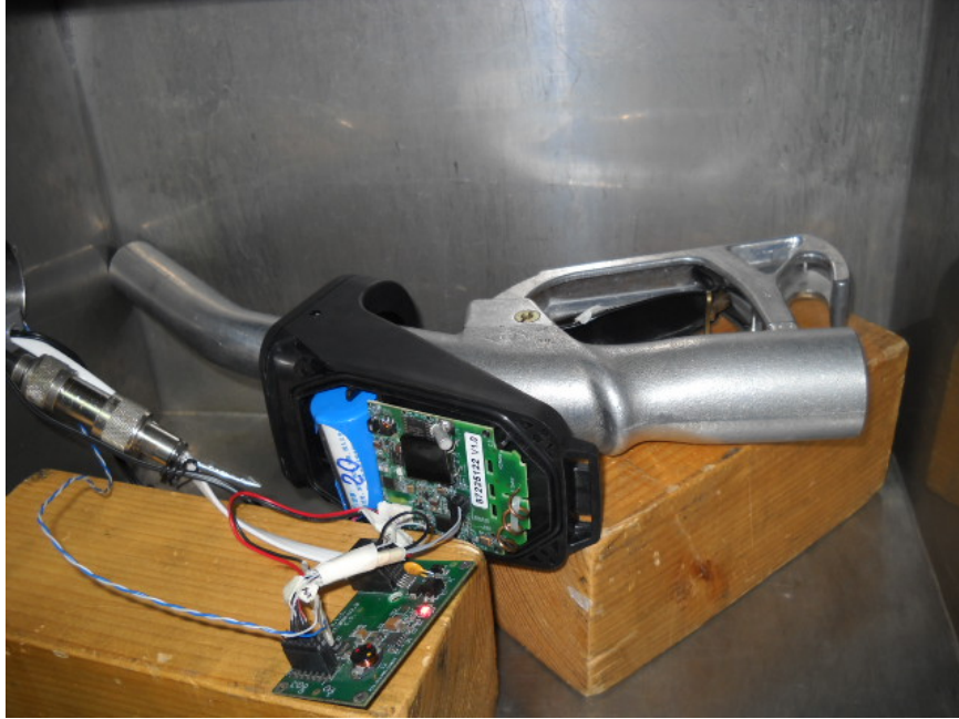
Photograph No.5 Frequency stability measurement setup
