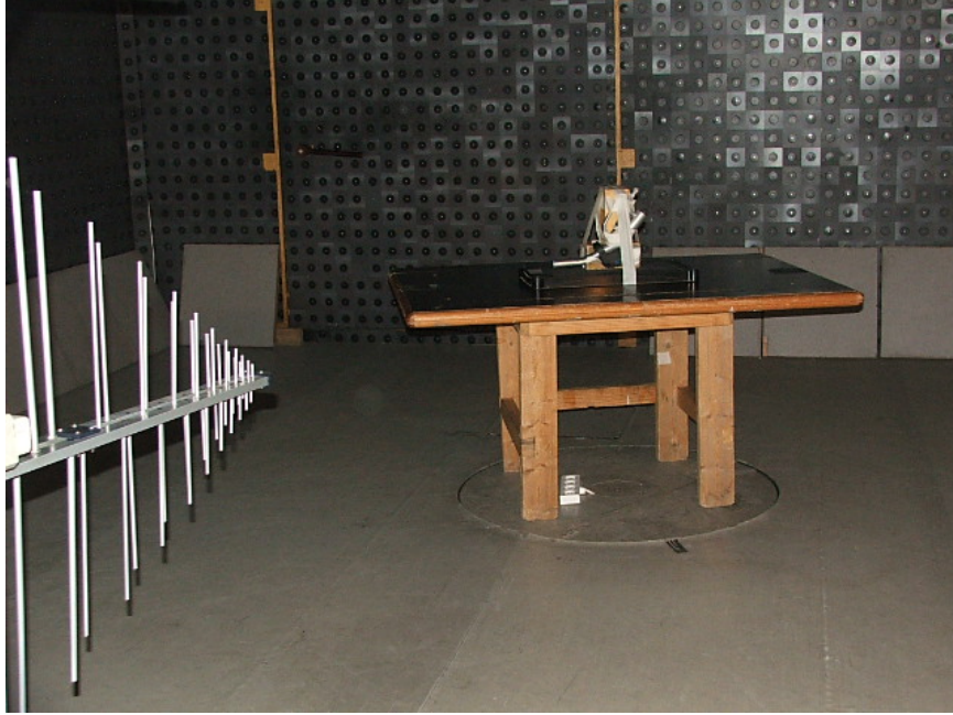
Photograph No.2 Radiated emissions measurement setup in the anechoic chamber in 30 – 1000 MHz
