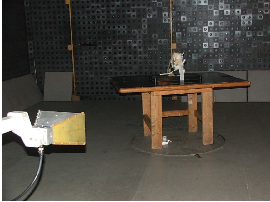
Photograph No.3 Radiated emissions measurement setup in the anechoic chamber above 1000 MHz
