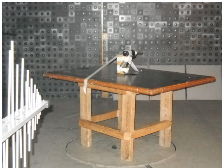
Photograph 8.1.1 Setup for radiated emission measurements
