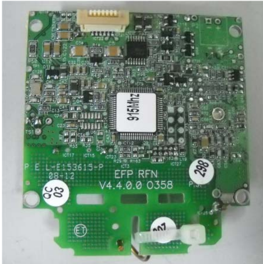
Photograph No.4 RF Nozzle reader PCB second side view
