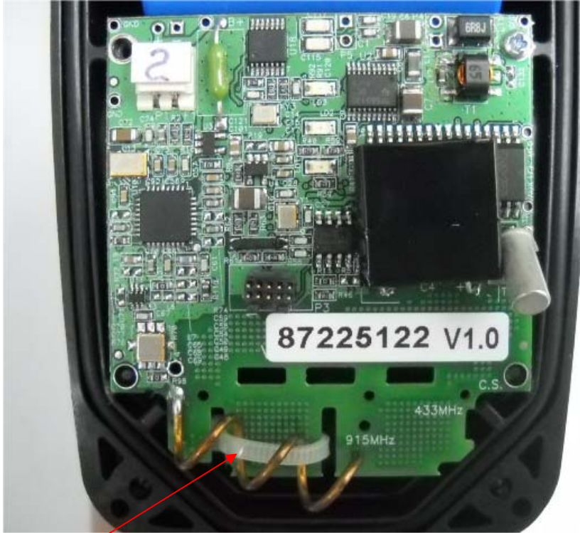
Site Controller antenna for 902-928 MHz range
