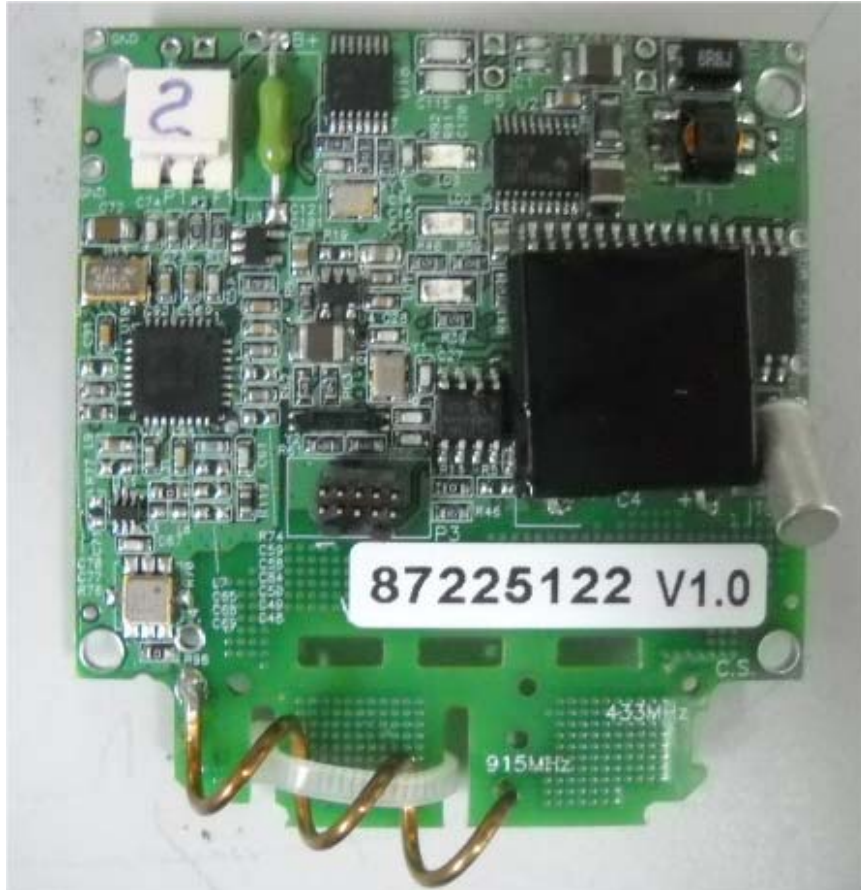
Photograph No.3 RF Nozzle reader PCB front view
