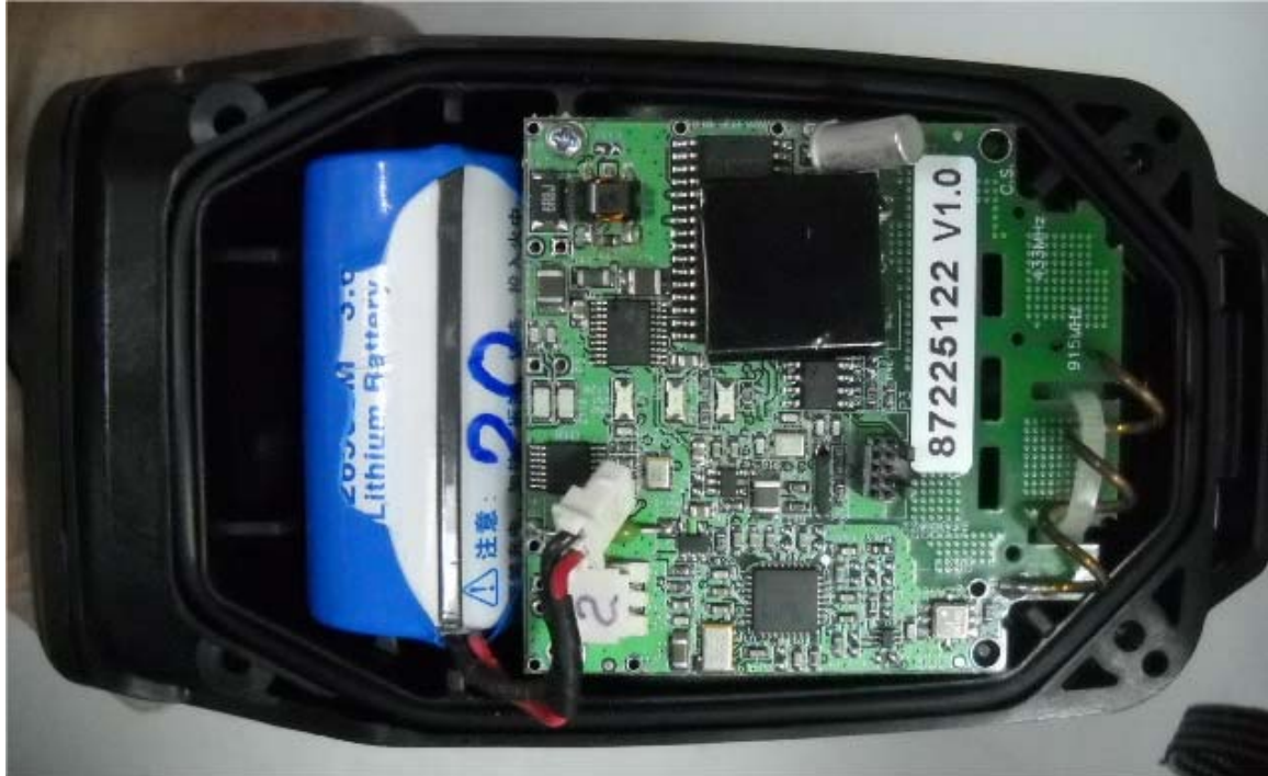
Photograph No.1 RF Nozzle reader internal view
