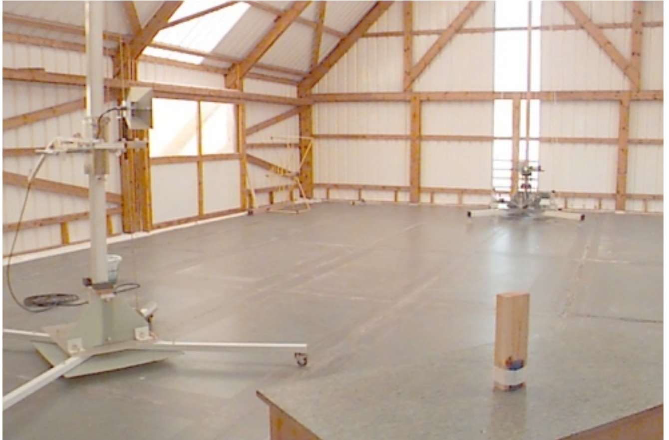
Photograph 1 Field strength of harmonics, OATS method
