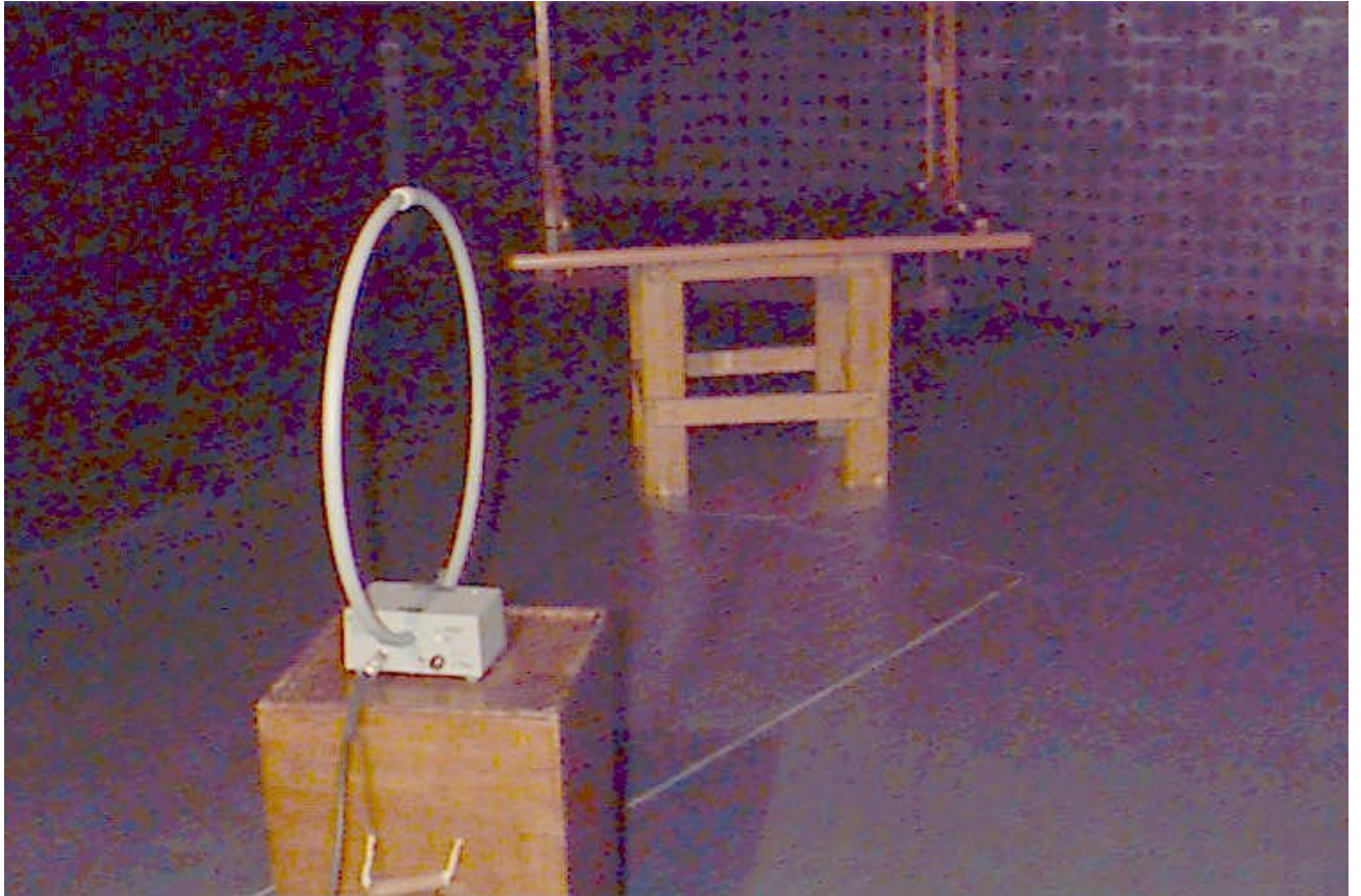
Photograph 2 Tx radiated emission measurements test setup with loop antenna, 9 kHz – 30 MHz frequency range, anechoic chamber method
