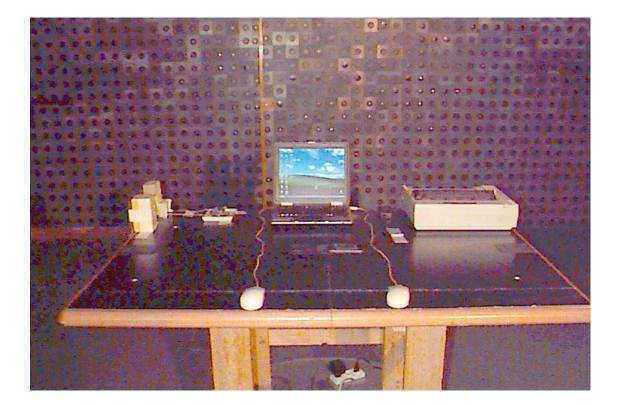
Photograph No.4 Radiated emissions measurement setup in the anechoic chamber
