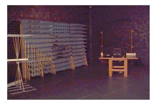
Photograph No.3 Radiated emissions measurement setup in the anechoic chamber
