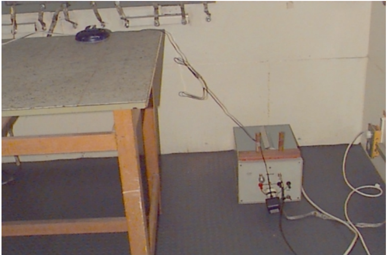
Photograph 4 Conducted emission measurements test setup
