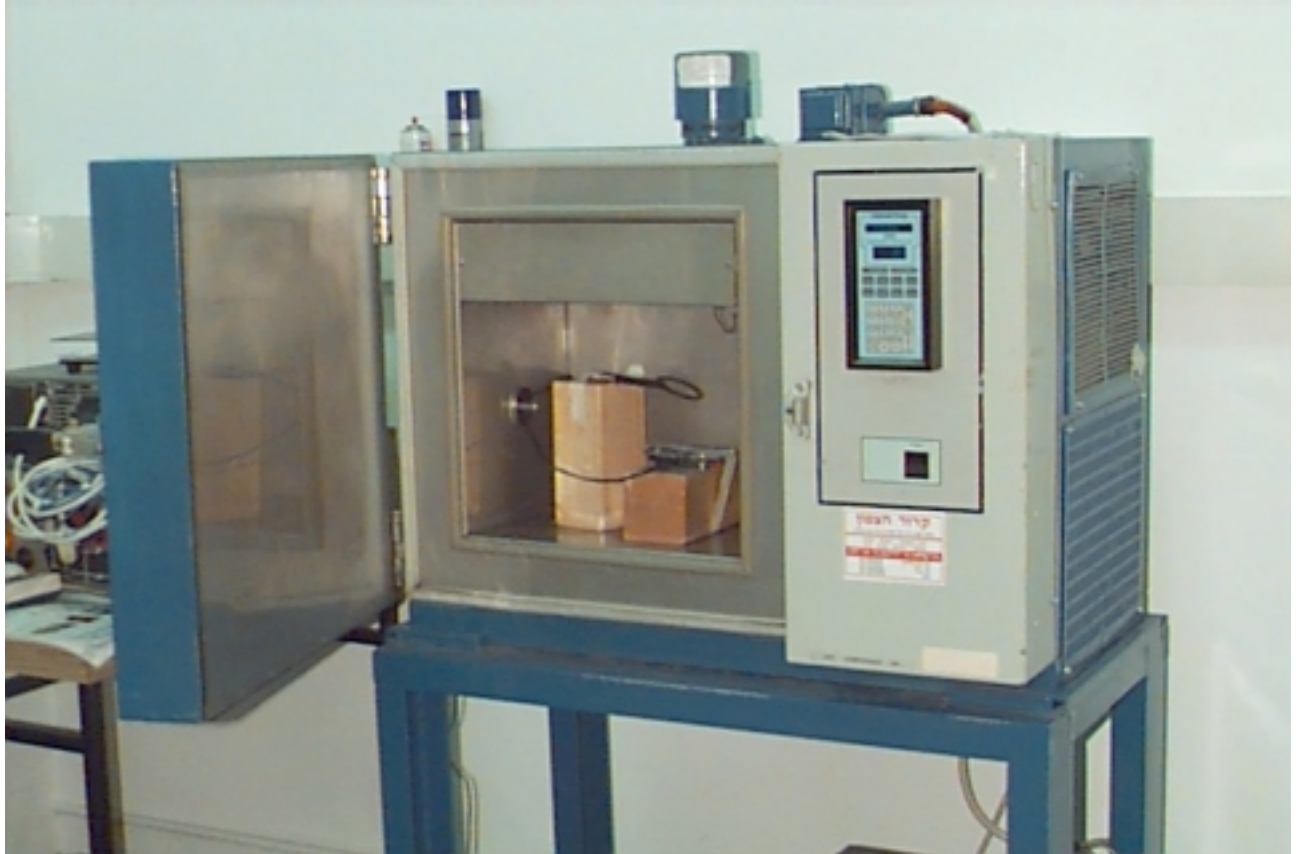
Photograph 6 Frequency tolerance test setup
