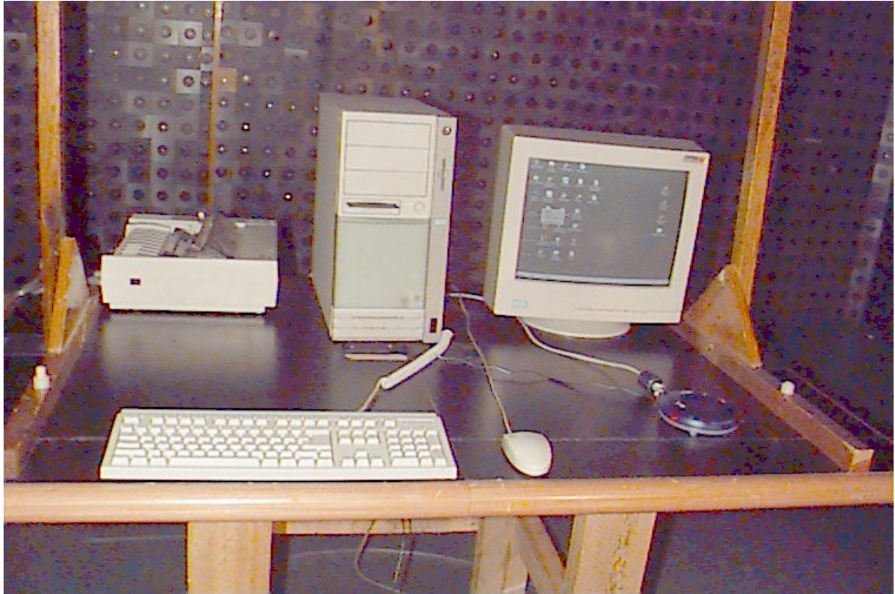
Photograph 4.2.2 Setup for radiated emission measurements The EUT view
