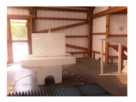
Photograph No.5 Radiated emissions measurement setup at the OATS above 1 GHz
