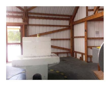
Photograph No.6 Radiated emissions measurement setup at the OATS above 1 GHz
