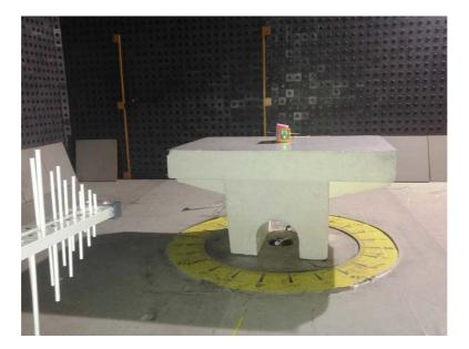
Photograph No.4 Radiated emissions measurement setup in the anechoic chamber above 1 GHz
