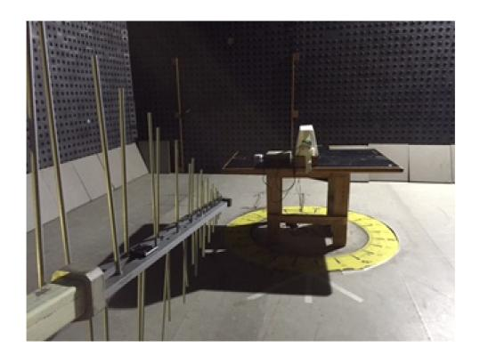
Photograph No.3 Radiated emissions measurement setup, EUT close view
