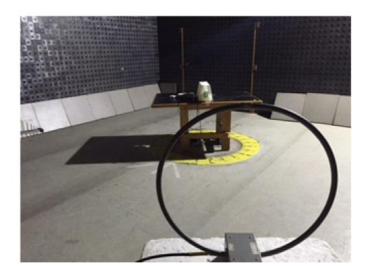
$\label{eq:Photograph No.2} Photograph No.2 \\ Radiated emissions measurement setup in the anechoic chamber in 30 – 1000 MHz$
