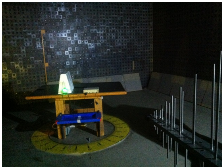
Photograph 8.2.1 Setup for preliminary radiated emission measurements
