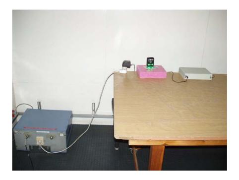
Photograph No.5 Setup for conducted emission measurement on AC power lines
