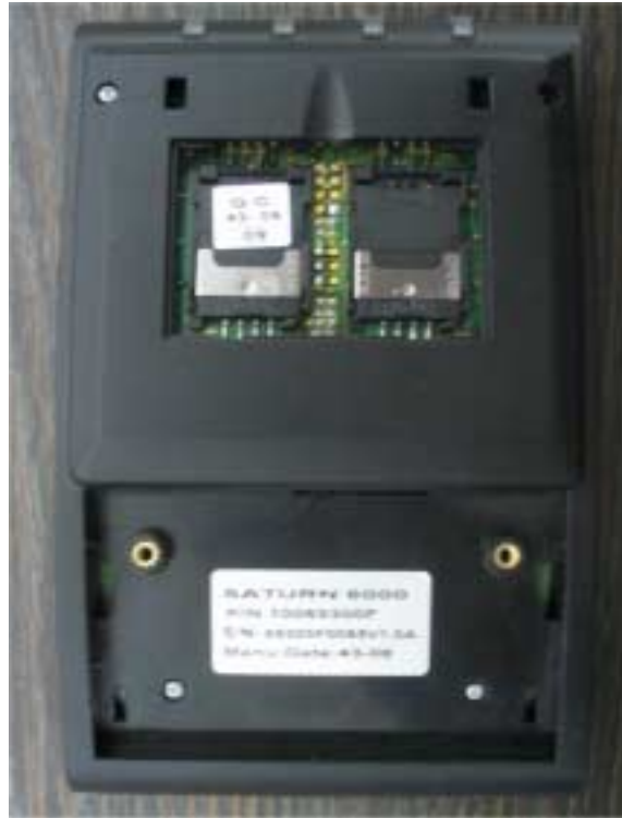
Photograph No.5 Card reader Saturn 6000 rear view without support
