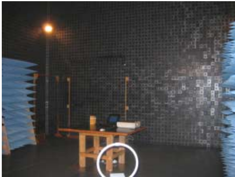
Photograph No.4 Radiated emissions measurement setup in the anechoic chamber with loop antenna, RS232 configuration
