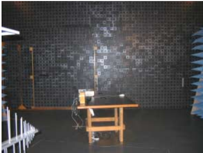
Photograph No.6 Radiated emissions measurement setup in the anechoic chamber with biconilog antenna, RS232 configuration
