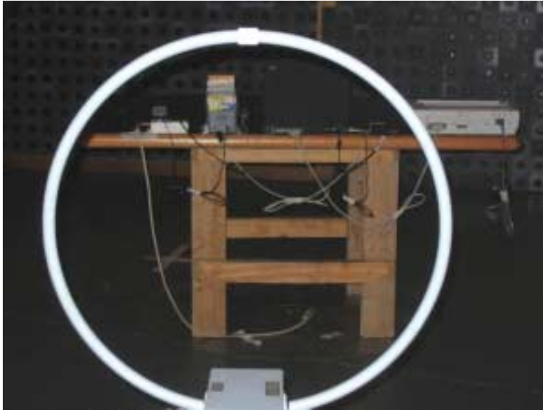
Photograph No.1 Radiated emissions measurement setup in the anechoic chamber with loop antenna, USB configuration
