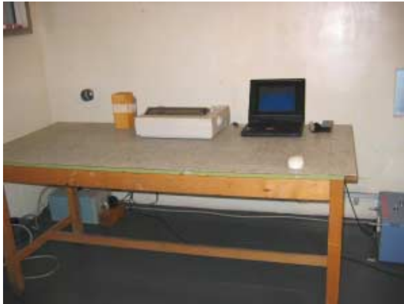
Photograph No.10 Conducted emissions measurement setup, RS232 configuration
