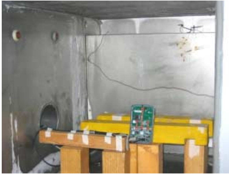
Photograph No.7 Frequency stability test setup, USB configuration
