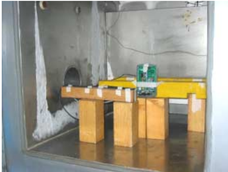
Photograph No.8 Frequency stability test setup, RS232 configuration
