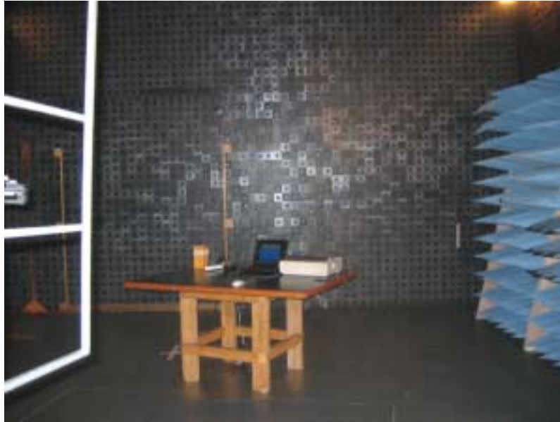
Photograph No.5 Radiated emissions measurement setup in the anechoic chamber with biconilog antenna, USB configuration
