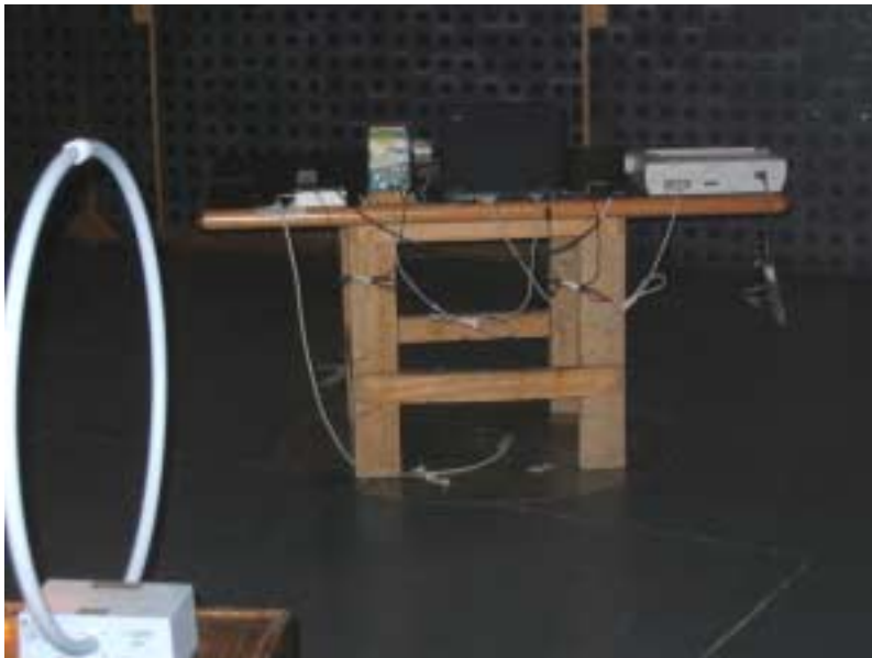
Photograph No.2 Radiated emissions measurement setup in the anechoic chamber with loop antenna, RS232 configuration
