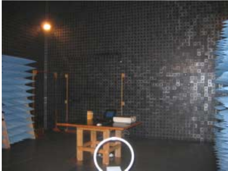
Photograph No.3 Radiated emissions measurement setup in the anechoic chamber with loop antenna, USB configuration
