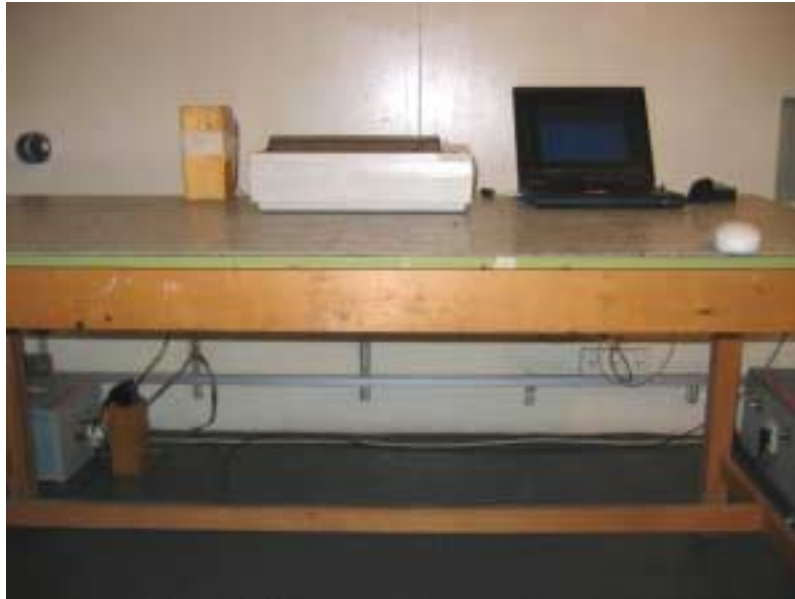
Photograph No.9 Conducted emissions measurement setup, USB configuration
