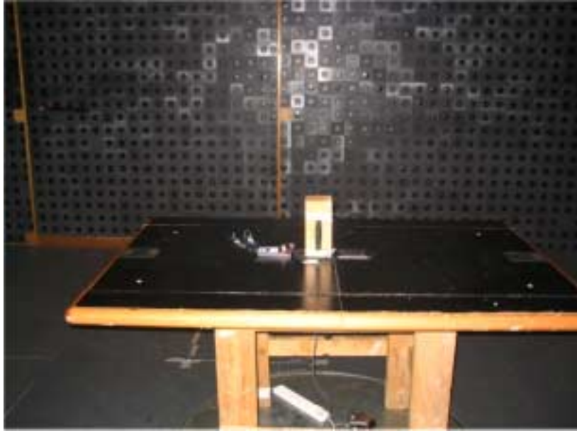
Photograph No.3 Fundamental and spurious emissions setup in the anechoic chamber, close view
