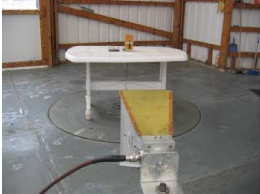
Photograph No.4 Spurious emissions measurement setup at the OATS with double-ridge guide antenna
