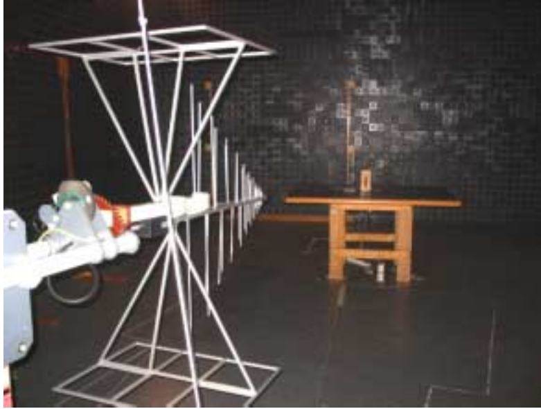
Photograph No.2 Field strength of fundamental and spurious emissions setup in the anechoic chamber with biconilog antenna
