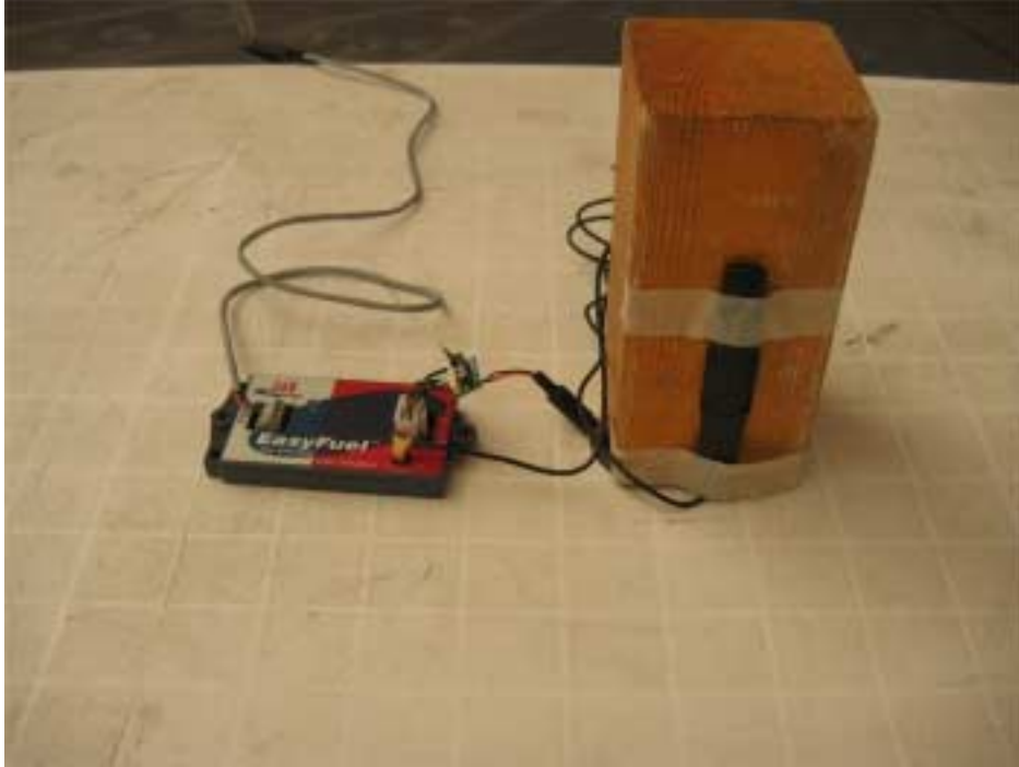
Photograph No.5 Spurious emissions measurement setup at the OATS, close view
