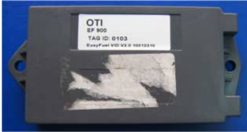
Photograph No.2 Vehicle identification unit rear view
