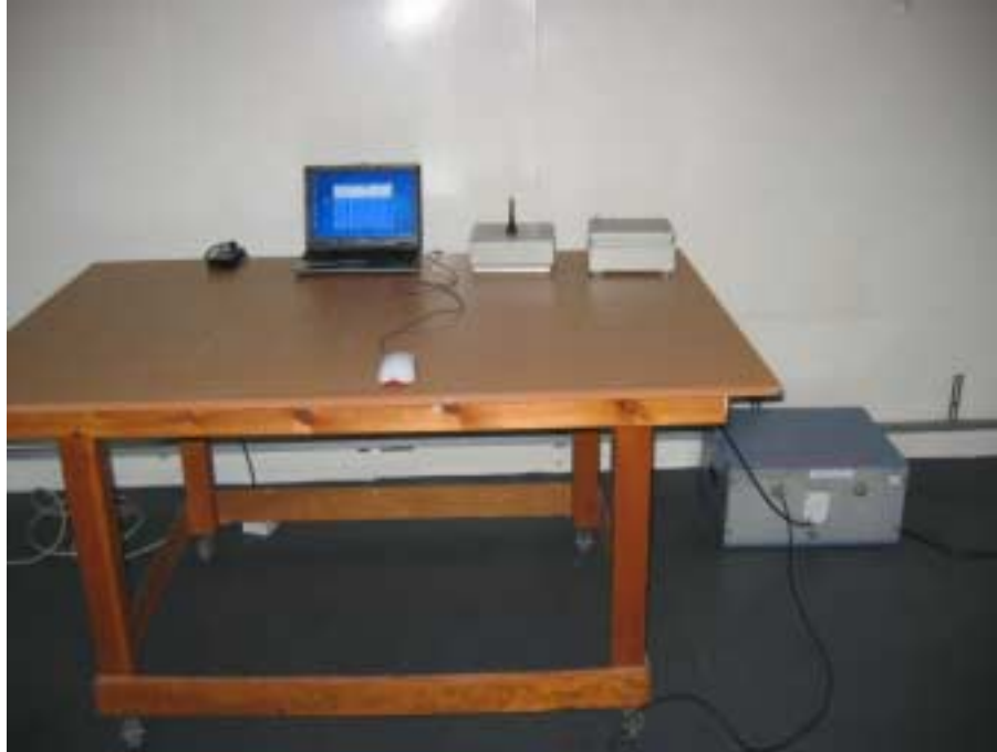
Photograph No.5 Conducted emissions measurement setup
