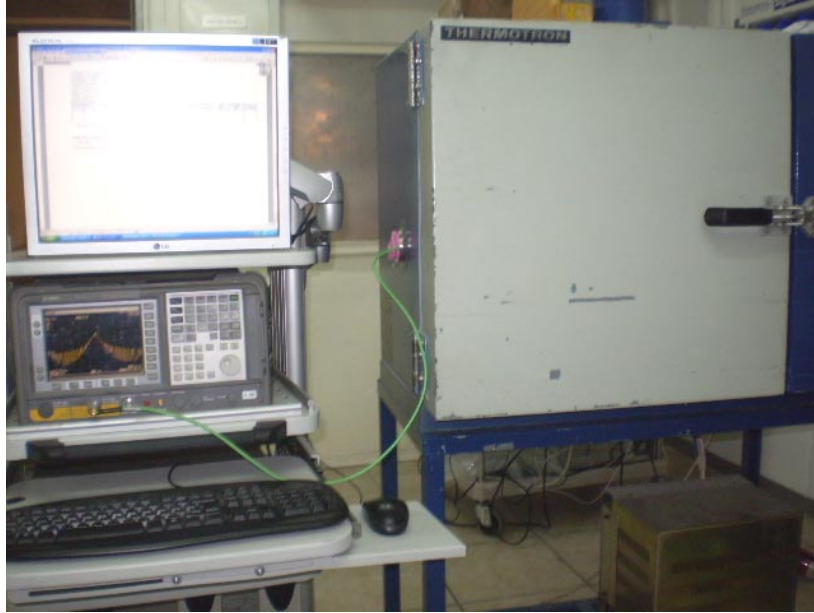
Photograph No.4 Frequency stability measurement setup
