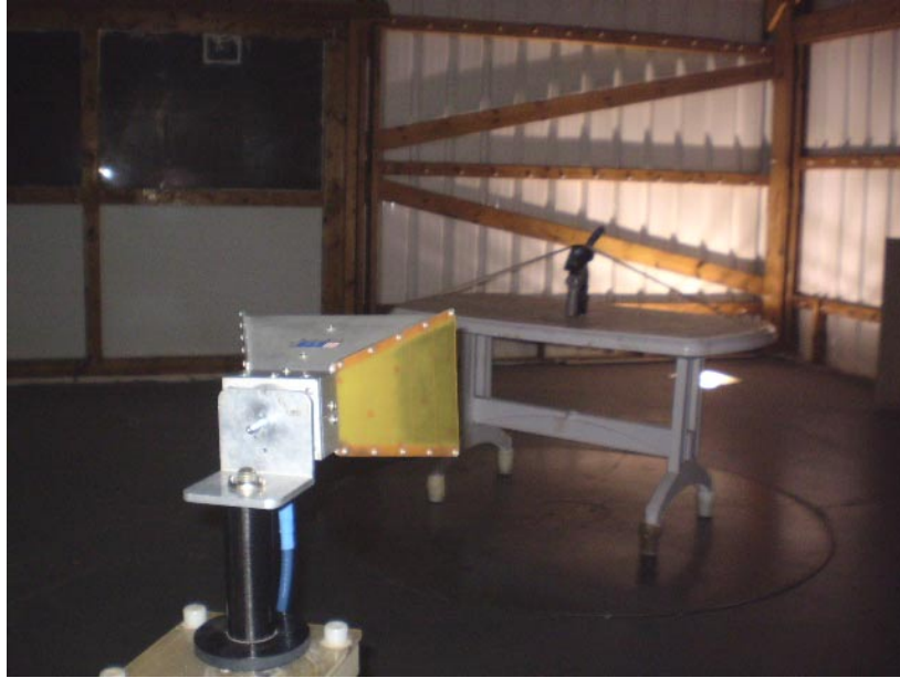
Photograph No.3 Radiated emissions measurement setup at the OATS above 1000 MHz
