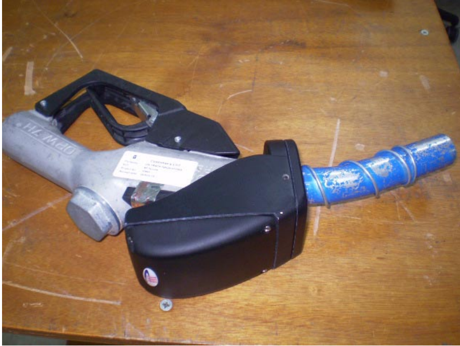
Photograph No.1 RF Nozzle reader front view
