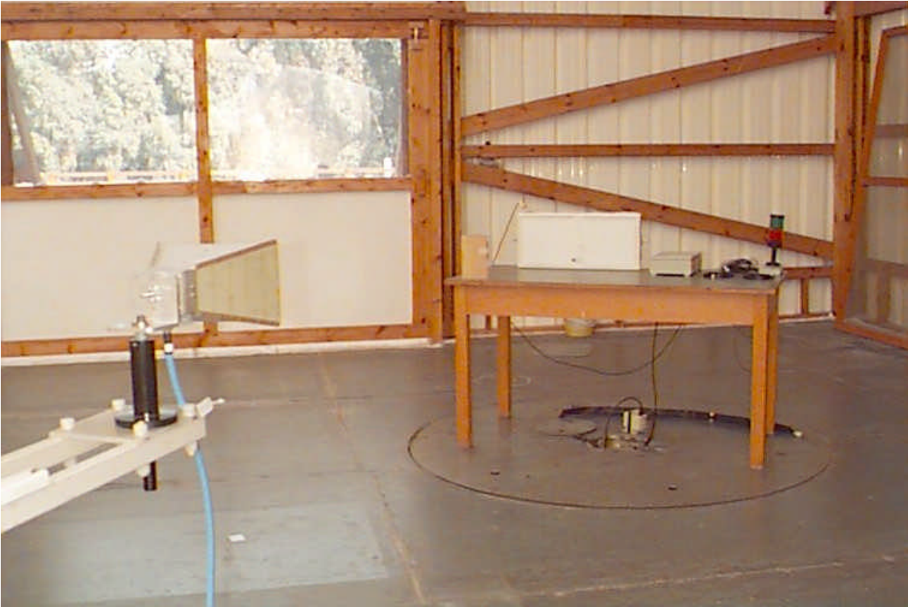
Photograph 10 Radiated emission measurements test setup with double ridge guide antenna, 5 GHz – 10 GHz frequency range, OATS method
