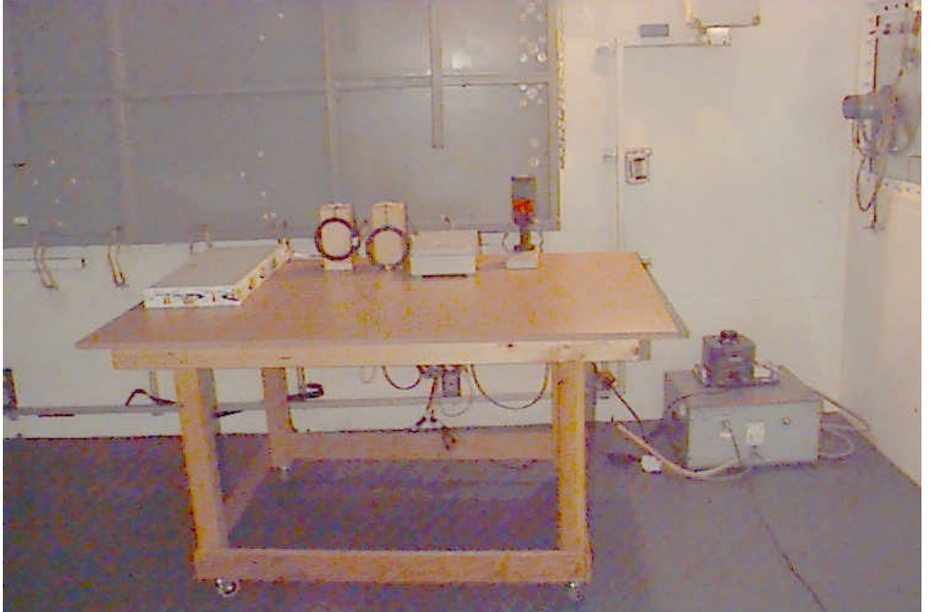
Photograph 11 Conducted emission measurements test setup
