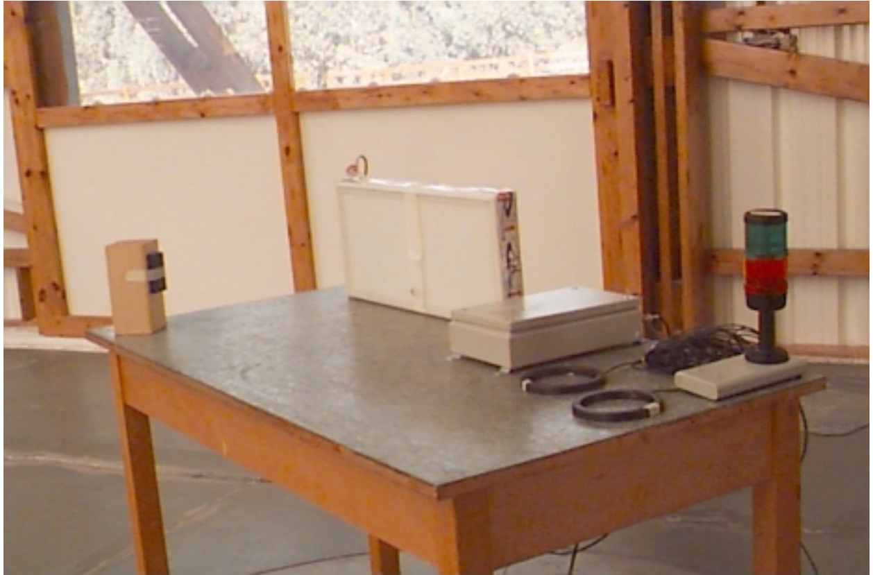
Photograph 9 Radiated emission measurements test setup with double ridge guide antenna, 5 GHz – 10 GHz frequency range, OATS method
