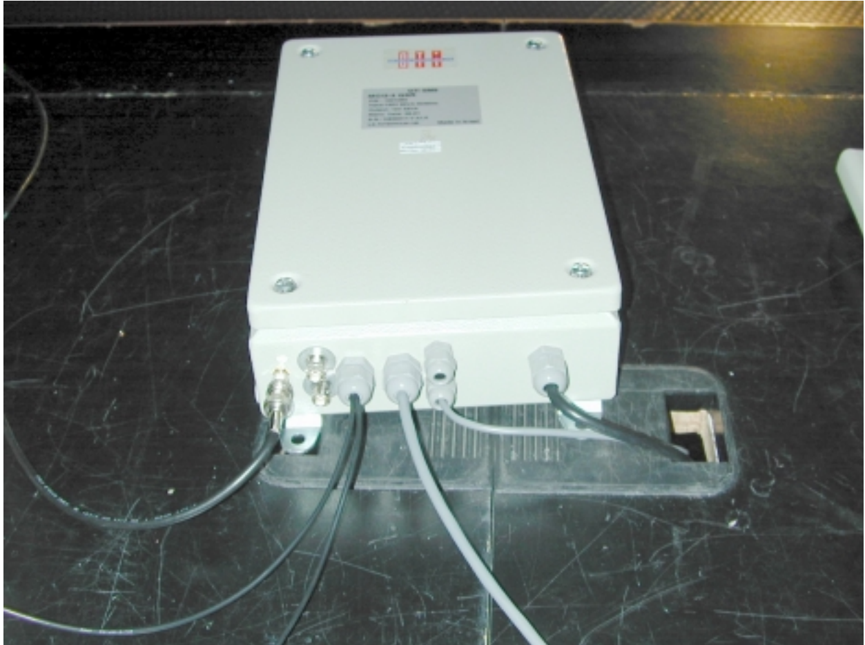
Photograph 4 Radiated emission measurements test setup with biconilog antenna, 30 MHz – 1000 MHz frequency range, anechoic chamber method
