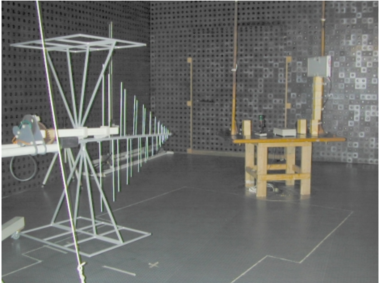
Photograph 2 Radiated emission measurements test setup with biconilog antenna, 30 MHz – 1000 MHz frequency range, anechoic chamber method
