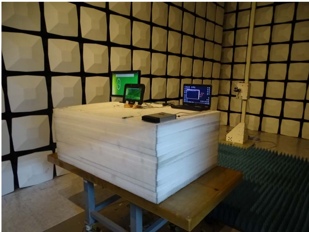
Back View of Radiated Test (Horn)
